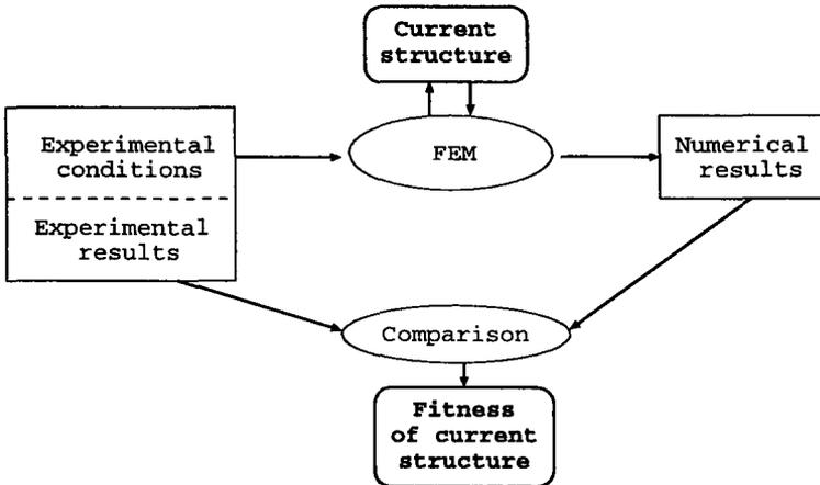
Figure 2: *Evolutionary approach for the inverse problem of mechanical inclusion identification: The fitness of the individual at hand is achieved by comparing the actual experimental results with the numerical results obtained by Finite Element Analysis on the structure that the individual represents.*
