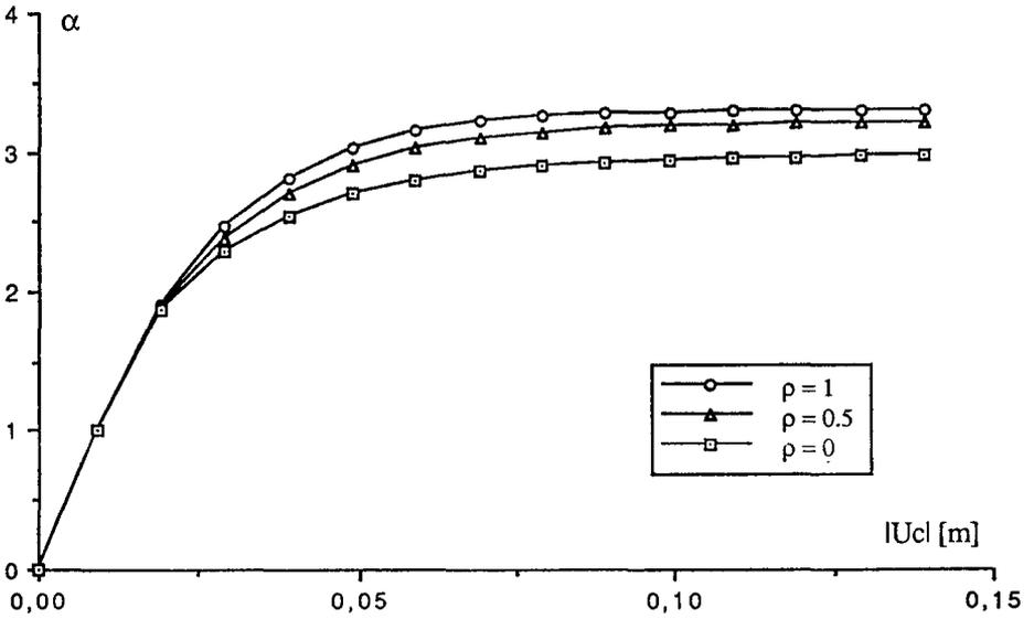
Figure 21. Load-displacement curves for the stability tunnel problem
