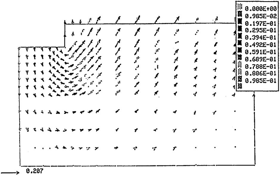
Figure 15. Failure mechanism for  $\phi = 20^\circ$  and  $\theta = 20^\circ$
