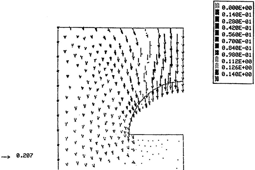
Figure 23. Failure mechanism for  $\varphi = 20^\circ$  and  $\theta = 10^\circ$
