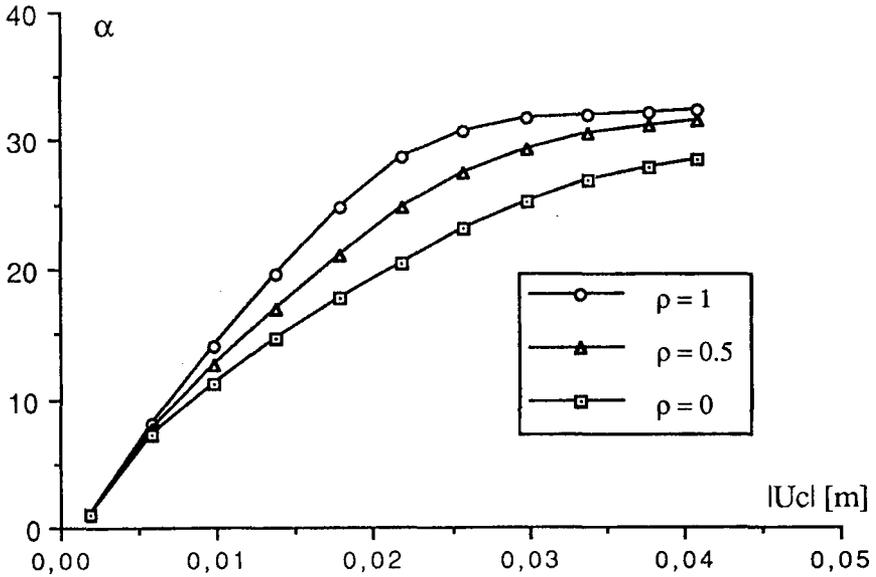
**Figure 14.** Load-displacement curves for the deep footing
