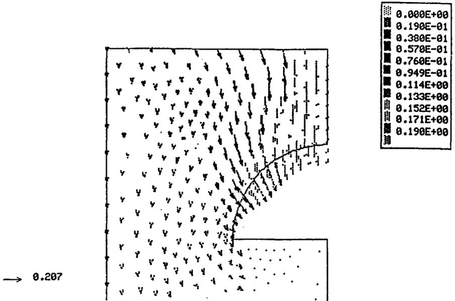
Figure 22. Failure mechanism for  $\phi = 20^\circ$  and  $\theta = 20^\circ$
