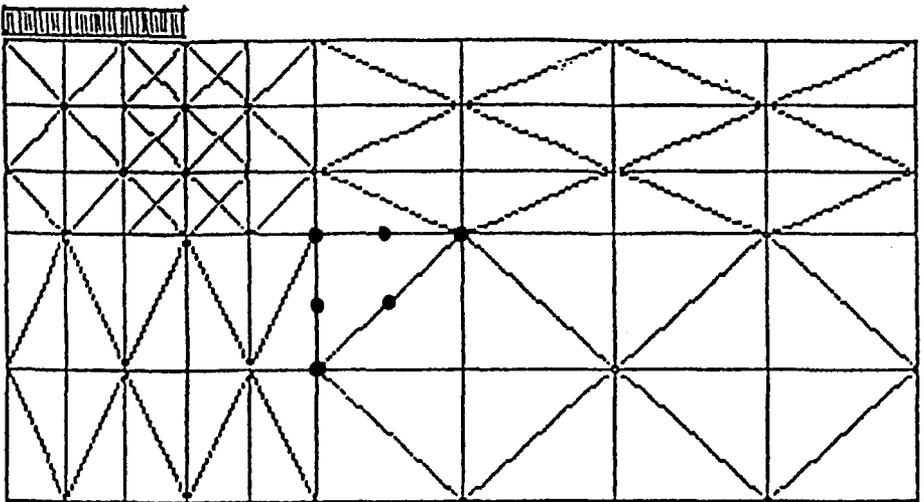
Figure 8. Meshe for the shallow strip footing
