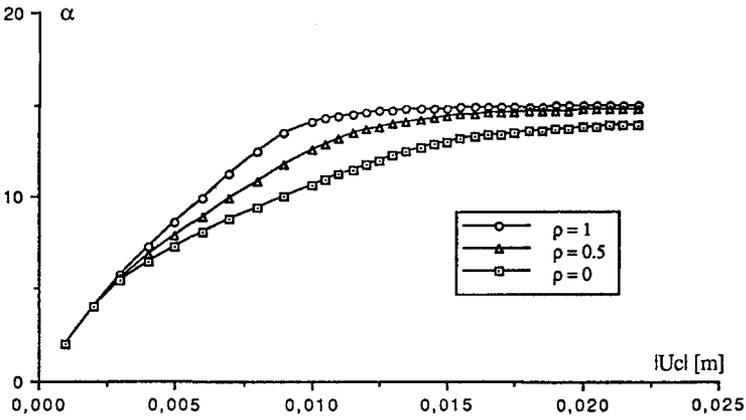
Figure 9. Load-displacement curves for shallow strip footing
