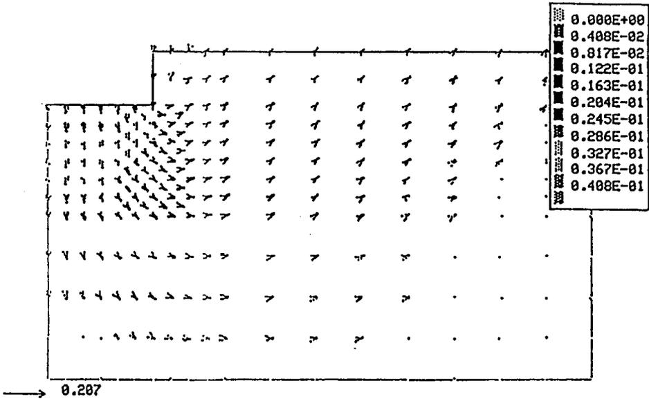
Figure 16. Failure mechanism for  $\phi = 20^\circ$  and  $\theta = 10^\circ$
