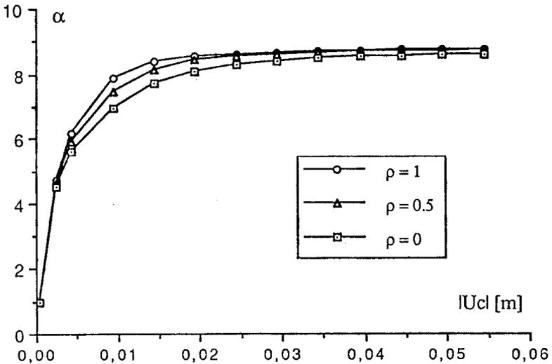
**Figure 17.** Load-displacement curves for the circular footing
