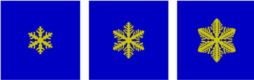
**Figure 6.** Effect of melting temperature  $T_m = .9, 1.0,$  and  $1.2$  (left to right) on dendrite.
