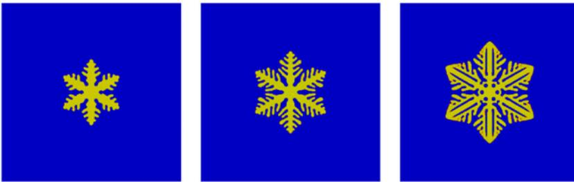
**Figure 8.** Effect of interfacial width  $\epsilon_0 = .009, .01, \text{ and } .011$  (left to right) on dendrite.
