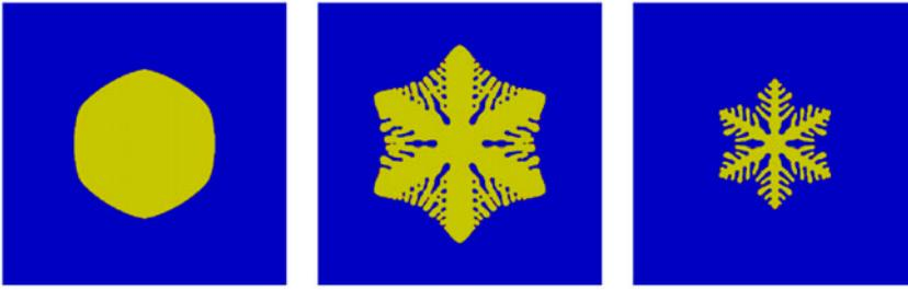
**Figure 5.** Effect of latent heat  $k = .5, 1.0,$  and  $1.8$  (left to right) on dendrite.
