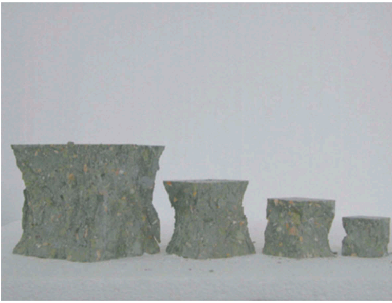
Figure 24. Crack patterns obtained in laboratorial experiments (Del Viso et al., 2008).
