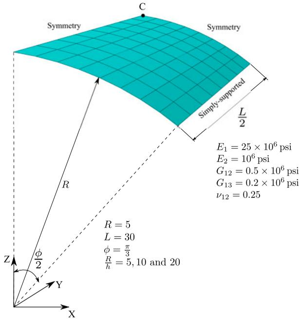
**Figure 4.** Simply-supported composite cylindrical panel meshed with  $8 \times 8$  quadrilateral shell elements.
