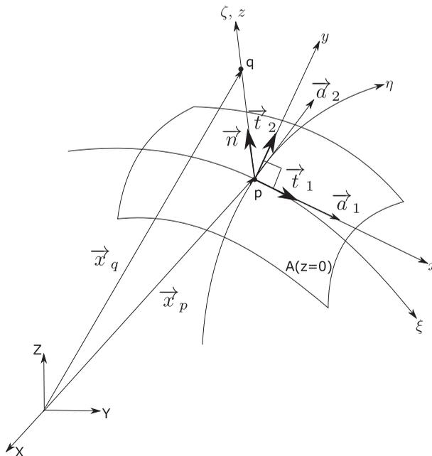
**Figure 1.** Geometry of a shell structure.
