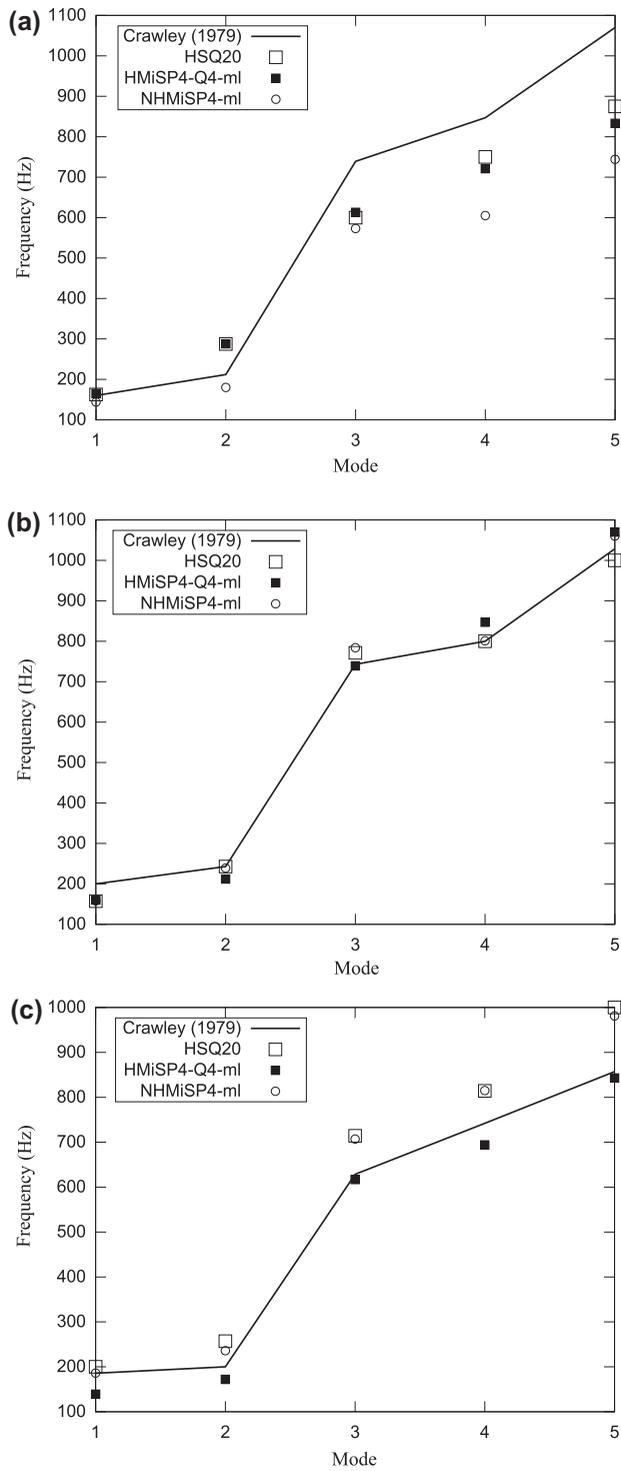
**Figure 6.** Natural frequencies of the clamped composite panels: (a)  $[0_2/\pm 30]_S$ , (b)  $[\pm 45]_{2S}$  and (c)  $[0/\pm 45/90]$ .
