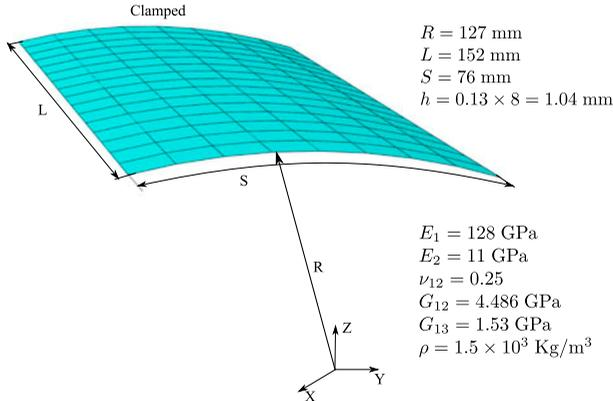
**Figure 5.** Cantilever composite panel meshed with  $8 \times 16$  quadrilateral shell elements.
