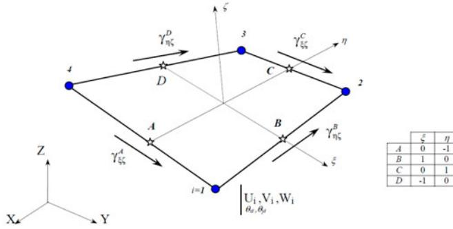
**Figure 3.** Projection of the covariant transverse shear strains.
