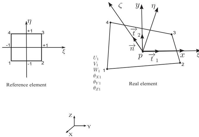
Figure 2. Four-node quadrilateral shell element.
