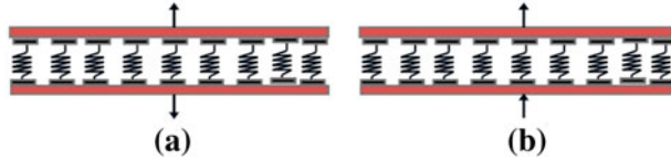
Figure 4. Special cases of the transverse motion of the elastically connected micro-panels: (a) asynchronous transverse motion; and (b) synchronous transverse motion.
