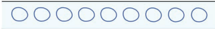
Figure 6 Snapshots of a capsule transported in a poiseuille flow field at equal time intervals. The capsule deforms into a egg shape at steady state.
