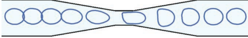
Figure 7 Snapshots of a capsule transported in a tapered channel at equal time intervals. The snapshots are close together at the entry of the narrow section indicating low speed whereas the speed increases at the exit of the constriction.
