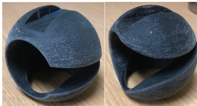
Figure 5 Actual 3D printed balls used for design 1 and design 2 valves.
