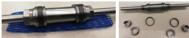
Figure 22 Piston with the seals and groove rings in an assembled (left) and disassembled (right) state (piston, seals, washers, screw nuts).
