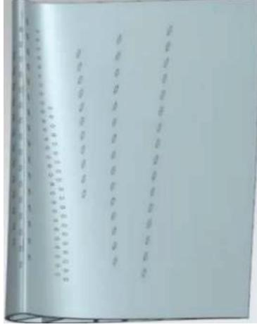
**Figure 4** Air film hole location.
