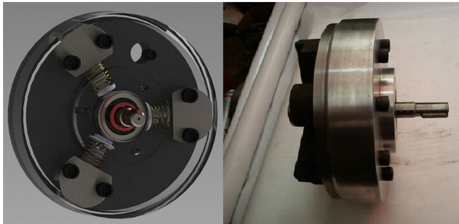
Figure 1. The designed and fabricated hydraulic piston pump.
