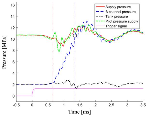
**Figure 8.** Opening response of valve number 3 in metering edge P-B.
