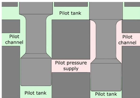
**Figure 3.** Position of the piloting spool when the solenoid is energised, i.e. main valve is opened (left side) and when a main valve is closed (right side).
