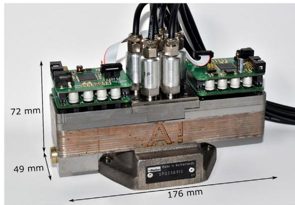
**Figure 6.** Valve system prototype mounted on an ISO 03 subplate.
