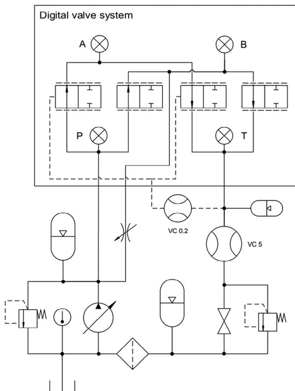
**Figure 5.** Hydraulic circuit of the valve test set-up.
