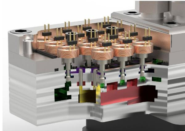
**Figure 2.** Cutaway view of the left half of the valve system.
