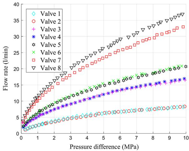
Figure 10. Flow rates of the valves in metering edge P-A.
