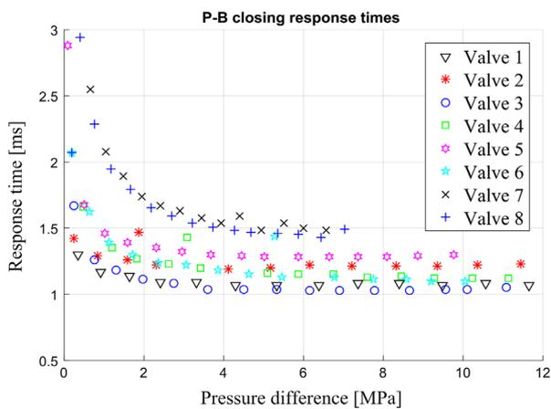
**Figure 9.** Closing response times of the valves in metering edge P-B.
