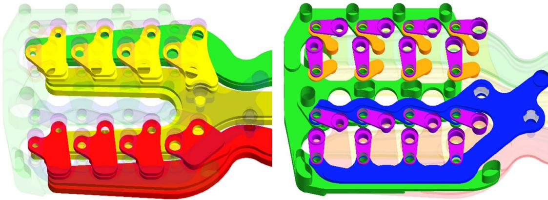
**Figure 4.** Flow channels inside the left half of the laminated manifold.
