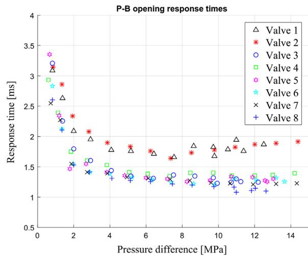
**Figure 7.** Opening response times of valves in metering edge P-B.
