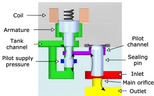
**Figure 1.** Cross section of a simplified model of one pilot operated on/off valve used in the valve system.
