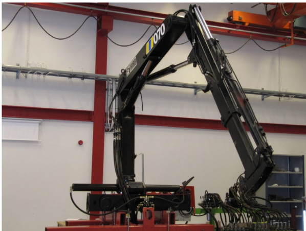
Figure 7. The crane used for experiments. The boom cylinder controls the first arm, the jib cylinder controls the second, telescope cylinders can extend the second arm and the swing cylinders can rotate the crane. The valve packages can be seen lower right.
