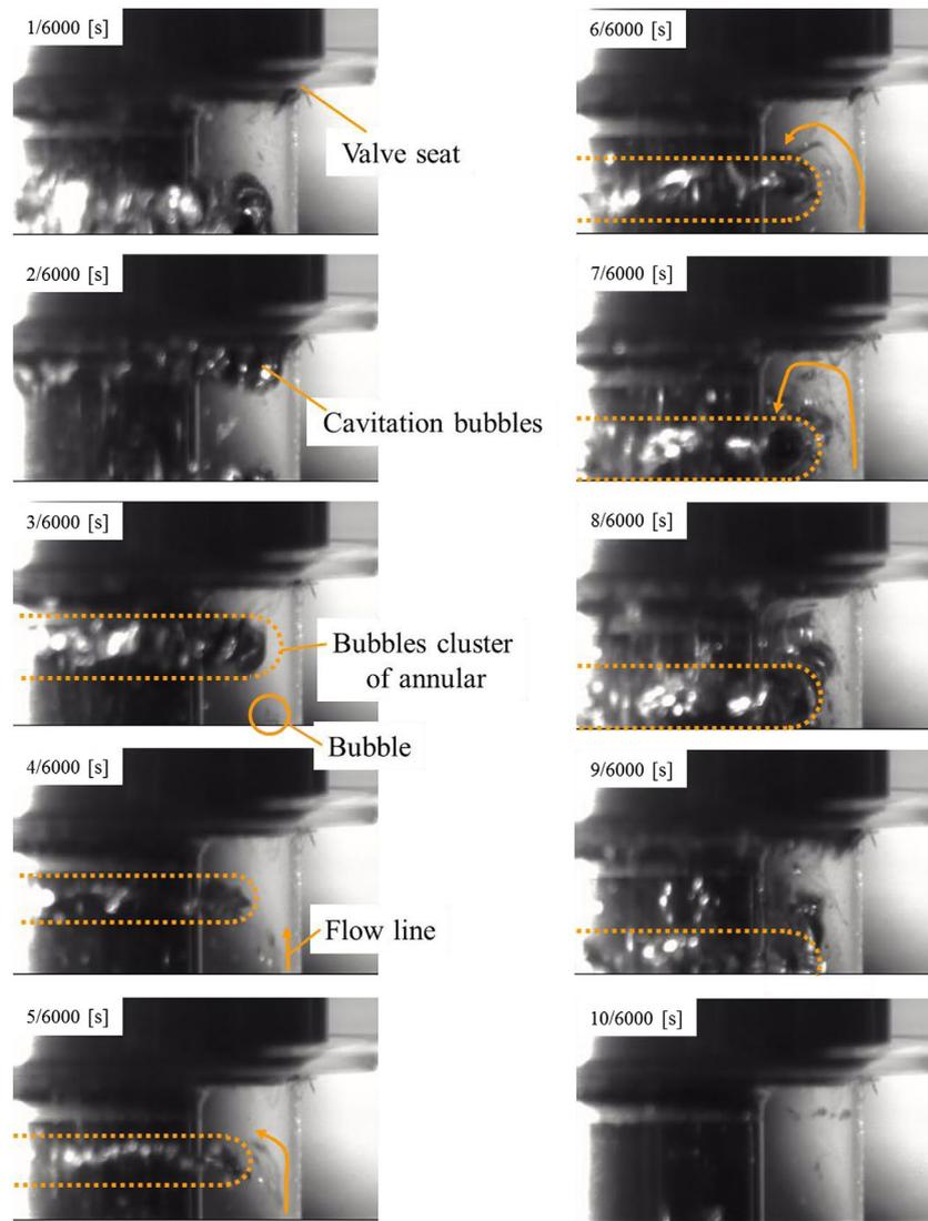
**Figure 4.** Flow state in downstream for  $Q = 10\text{ L/min}$  and  $T = 30\text{ }^\circ\text{C}$ . These images are the portion A in Figure 3.
