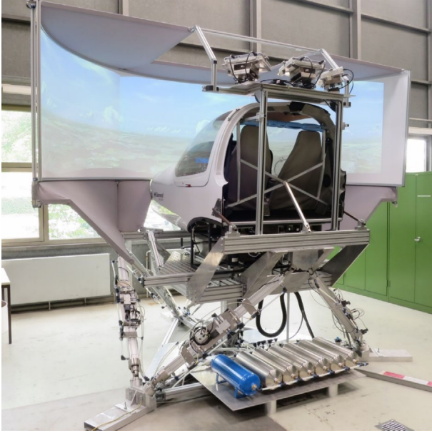
Figure 3. Pneumatically actuated motion platform for a full flight simulator, “Project ServoFlight” at the Institute for System Dynamics, University of Stuttgart.
