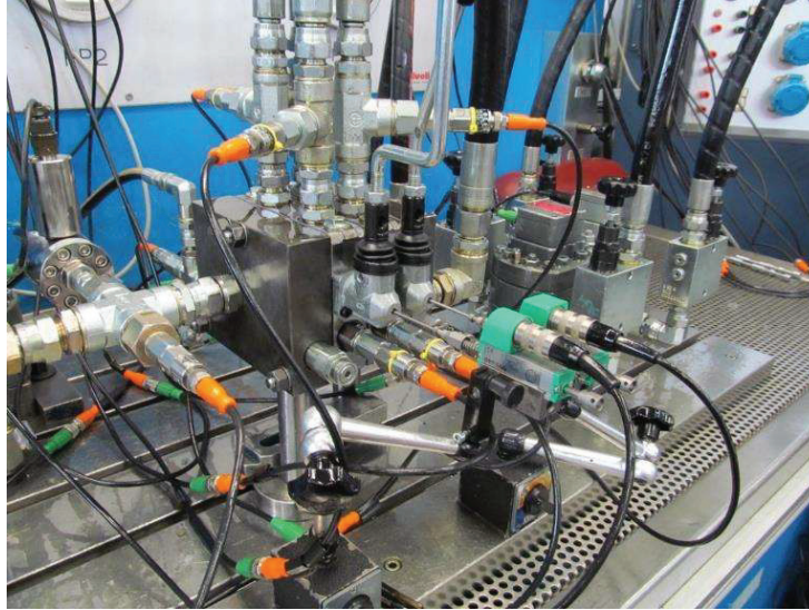
Figure 5 Prototype of two sections DCV on test bench.
