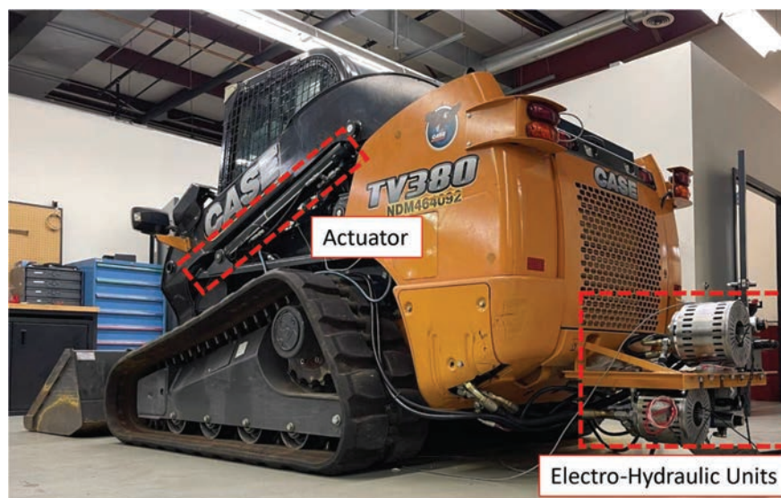
Figure 3 Electro-hydraulic units mounted on the reference machine and connected to the actuators.
