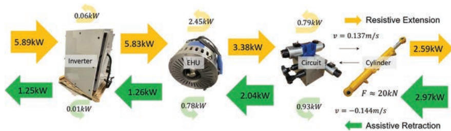
Figure 16 Power flow of the proposed EHA, extension, and retraction with 20 kN load.
