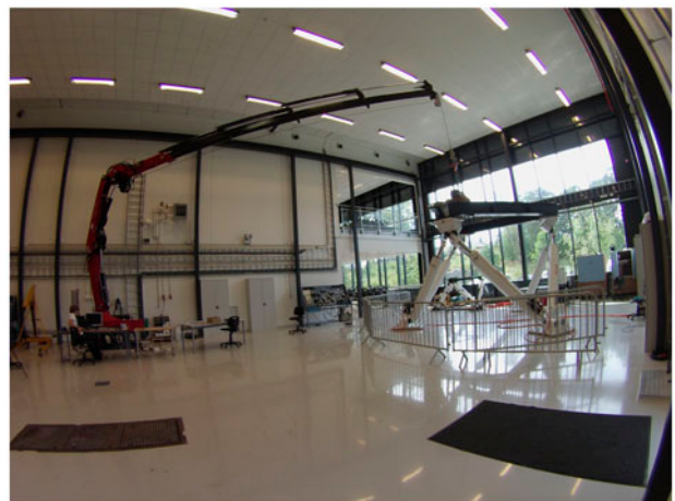
Figure 10. Photo of the vehicle loader crane located in the motion laboratory.
