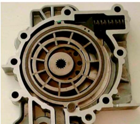
Figure 17. Crankshaft mounted vane pump – rotational stator.
