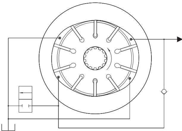
Figure 27. Balanced vane pump.
