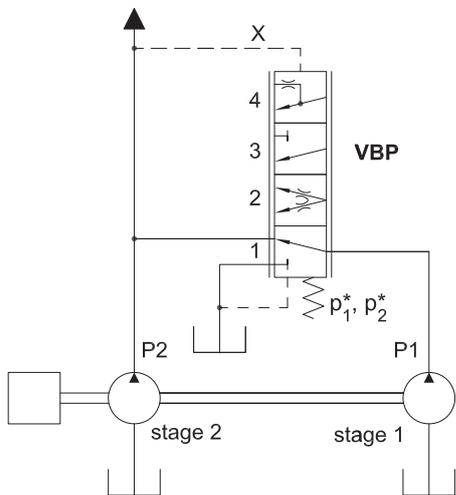
Figure 23. Hydraulic circuit of a dual-stage gerotor pump.
