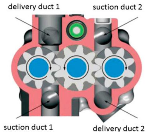
Figure 25. Dual-delivery external gear pump (Voigt, 2011).
