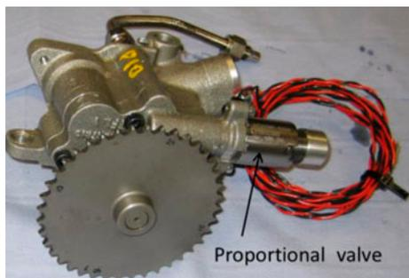
Figure 40. Pump with proportional control (Burke *et al.* 2012).
