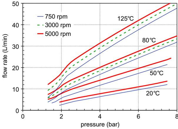
Figure 1. Flow-pressure curves of a lubricating circuit.
