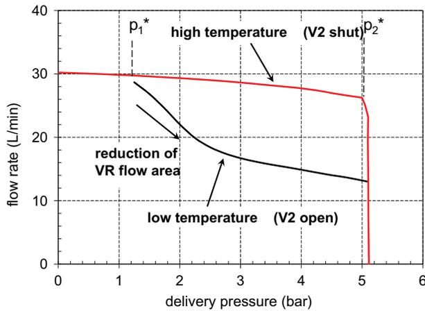
Figure 37. Characteristics with thermostatic control.
