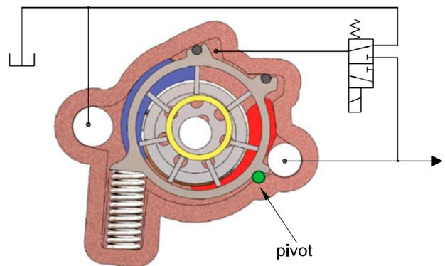
Figure 39. Alternative solution of two level electric control.
