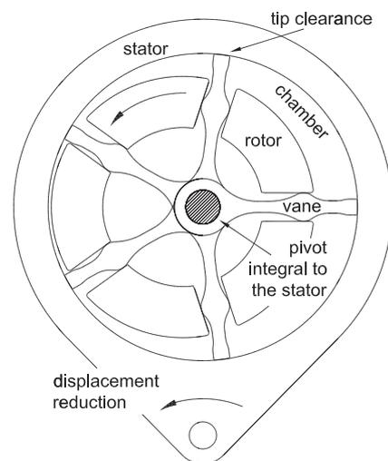
Figure 21. Central-vane pump.
