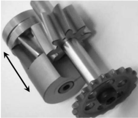
Figure 22. Sliding gears pump (Voigt, 2003).
