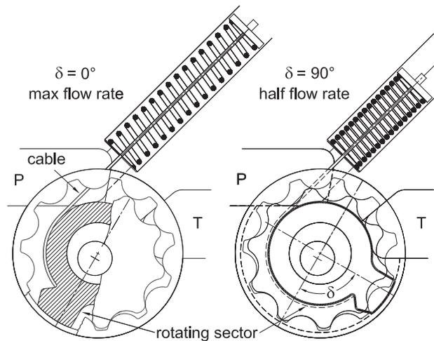
Figure 29. Prototype of variable timing pump.
