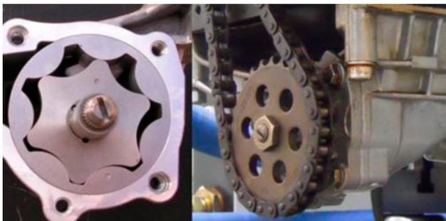
Figure 5. Off-axis gerotor lubricating pump.
