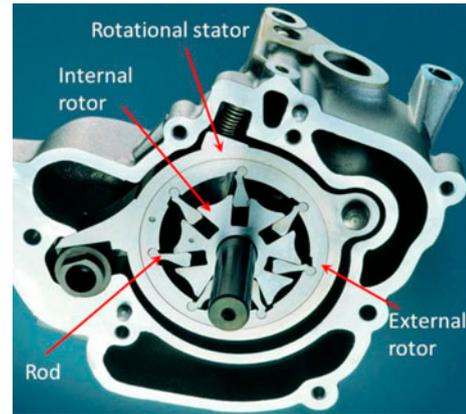
Figure 20. Pendulum pump.
