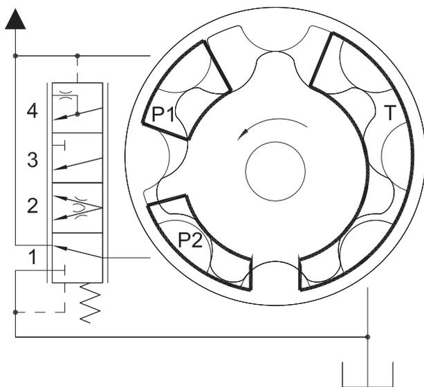
Figure 31. Discrete variable timing principle.
