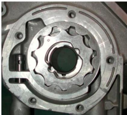
Figure 4. Gerotor lubricating pump.
