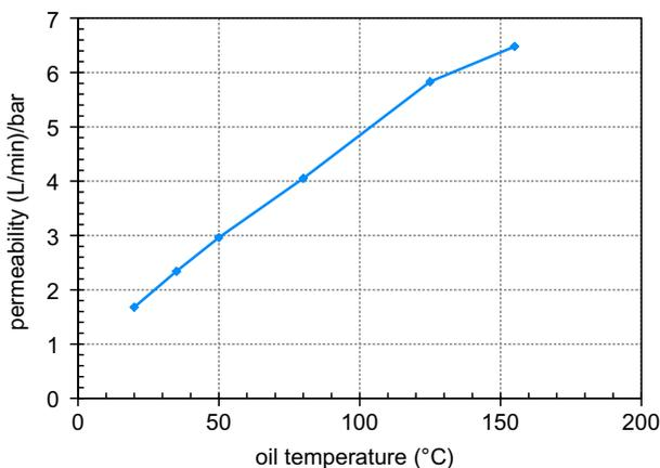
Figure 2. Typical circuit permeability vs. temperature.
