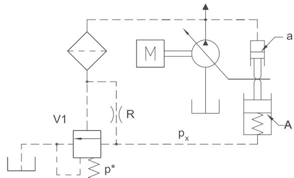
Figure 18. Piloted variable displacement pump.
