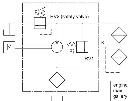
Figure 8. Flow generating unit with external pilot.
