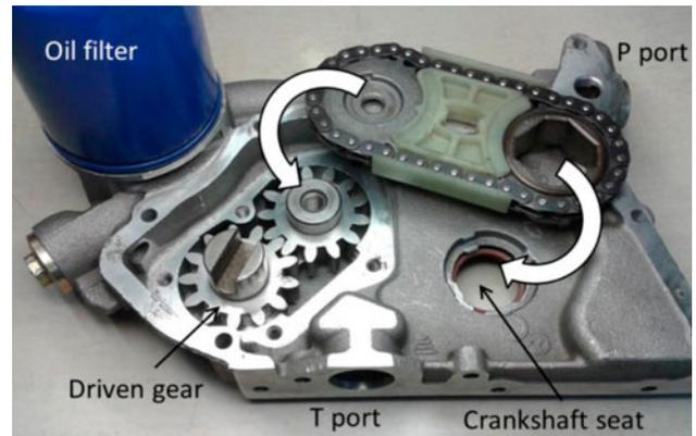
Figure 7. External gear pump.
