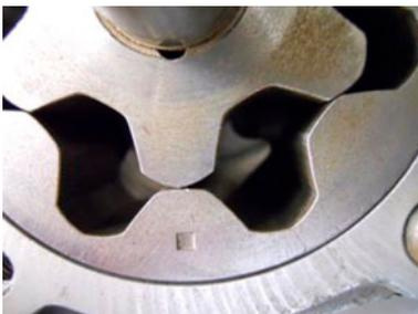
Figure 13. Detail of the Duocentric profiles.
