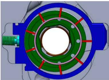
Figure 16. Crankshaft mounted vane pump – translational stator.
