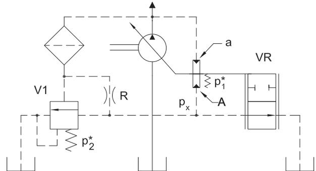
Figure 35. Principle of two fixed levels pressure control.
