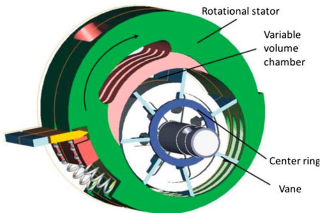
Figure 19. Alternative solution for rotational stator (Neukirchner *et al.* 2002).
