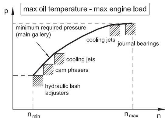
Figure 3. Minimum required pressure vs. engine speed.
