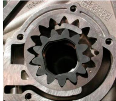
Figure 6. Crankshaft mounted crescent pump.
