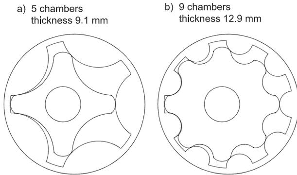
Figure 12. Gears with different profiles.
