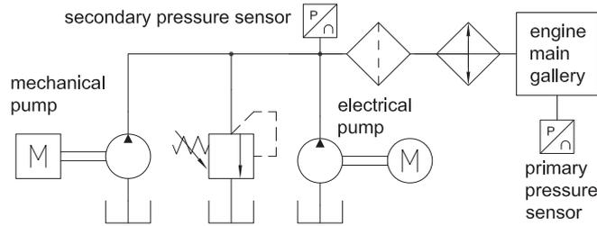
Figure 33. Layout with electric pump.
