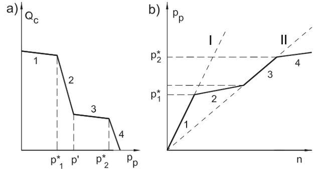
Figure 24. Characteristics of a dual stage pump.
