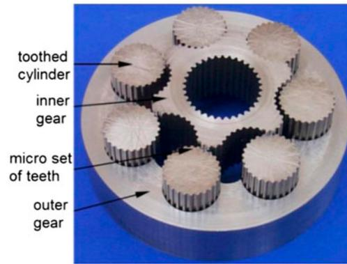
Figure 14. Gears with micro set of teeth (Bachmann *et al.* 2000).
