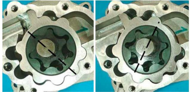
Figure 28. Variable timing gerotor pump.
