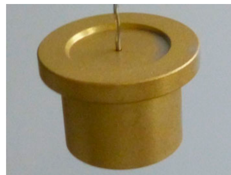
Figure 3. Pristine sample made in \text{CuZn}_{40}\text{Al}_2 alloy.
