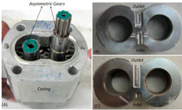
Figure 16. (A) Prototype optimal gears assembled within the commercial casing. (B) Lateral bushings with grooves for max. (100%) displacement. (C) Lateral bushings with grooves for min. (68%) displacement.
