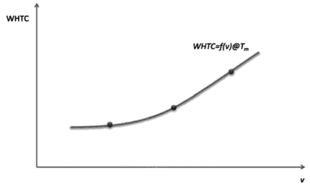
Figure 10. Cubic spline of the WHTC as a function of velocity for a given temperature t_m .
