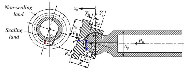
Figure 2. The free body diagram of a piston assembly.
