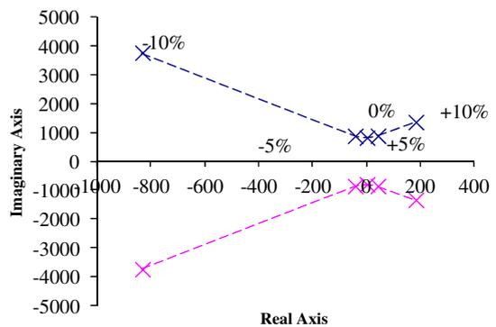
Figure 7. Poles movement by  $r_s$ .
