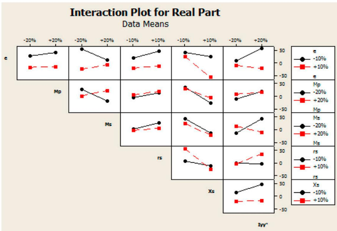
Figure 10. Interactions of the real part of poles by design parameters.
