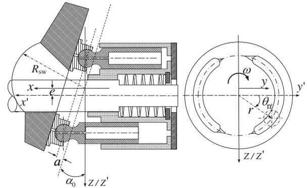
Figure 1. The schematic of an axis piston pump.
