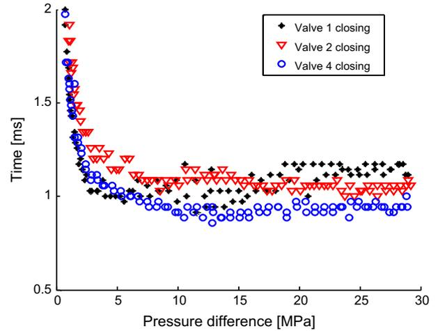
Figure 8. The closing response times of valves 1, 2 and 4 as a function of the pressure difference.
