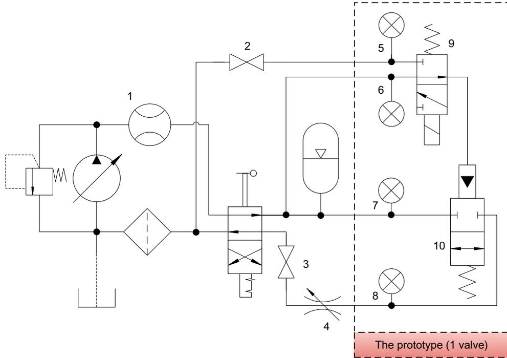
Figure 3. The hydraulic circuit of the test setup.
