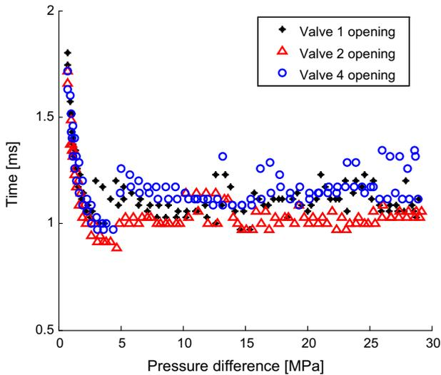
Figure 7. The opening response times of valves 1, 2 and 4 as a function of the pressure difference.
