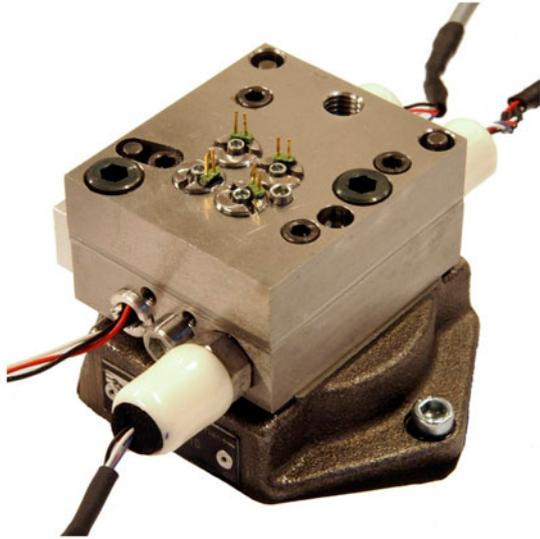
Figure 2. The four-valve prototype mounted on a CETOP 3 subplate.
