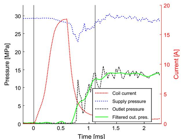
Figure 5. The pressures and the coil current of valve 4 during an opening cycle.
