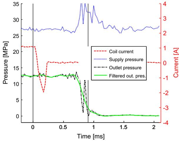
Figure 6. The pressures and the coil current of valve 4 during a closing cycle.
