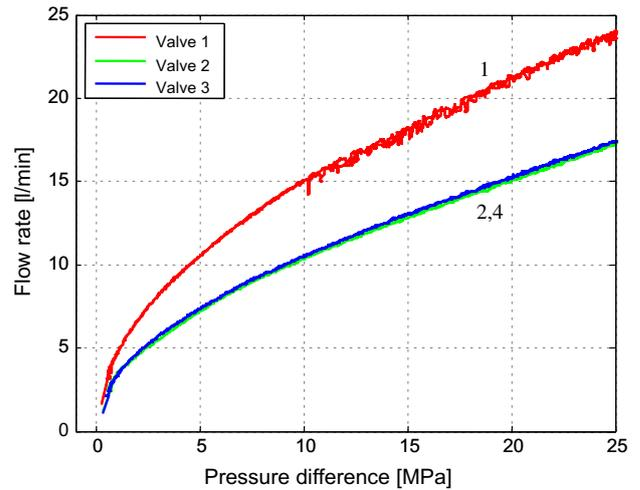
Figure 4. The flow rates through the valves as a function of the pressure difference.
