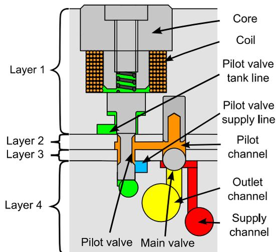
Figure 1. Cross section of the designed valve when the solenoid is not energised i.e. the main valve is in closed state. Figure not in scale.
