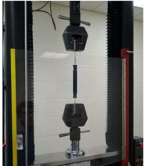
Fig. 9: Polyurethane of durometer 40A uniaxial tensile test with same specimen to be used in DPEA testing
