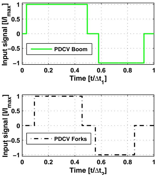
Fig. 22: Boom and forks PDCV commands ( $\Delta t_1=26s$ ,  $\Delta t_2=19s$ )
