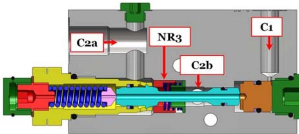
Fig. 9: Section view of OVC3 valve
