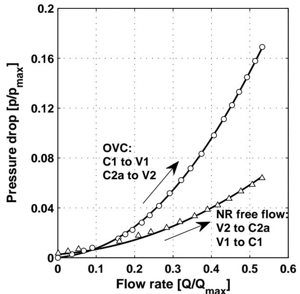
Fig. 16: Comparison between simulated and experimental pressure drop at maximum opening (For  $Q_{max}$  and  $p_{max}$  values refer to Table 2)
