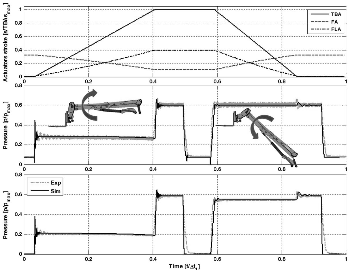
Fig. 24: Actuators stroke(top) Pump delivery pressure P4 (middle); Load Sensing pressure P5 (bottom)
