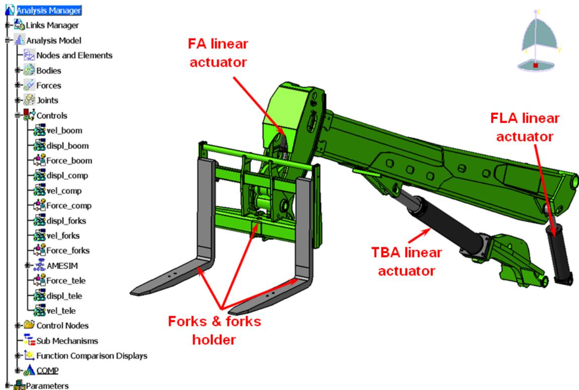
Fig. 20: Virtual Lab Motion telescopic boom model
