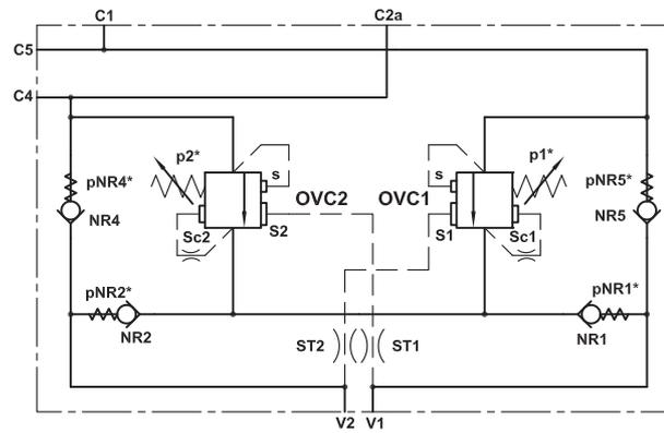
Fig. 14: ISO scheme of dual OVC valve
