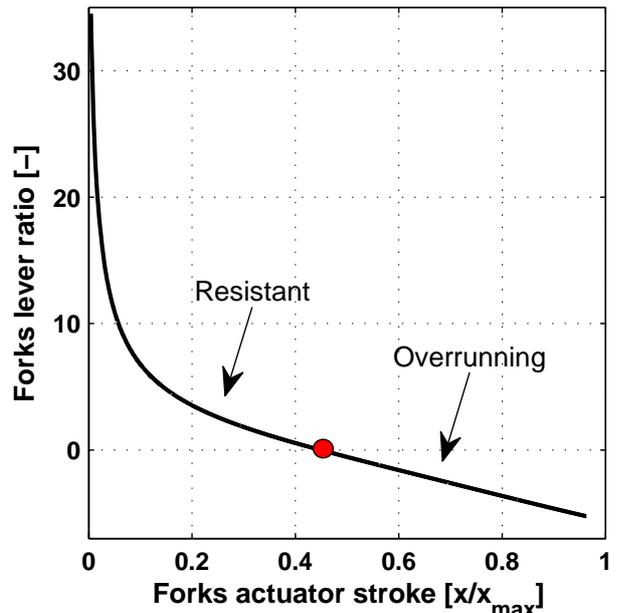
**Fig. 6:** Forks lever ratio vs. forks actuator stroke
