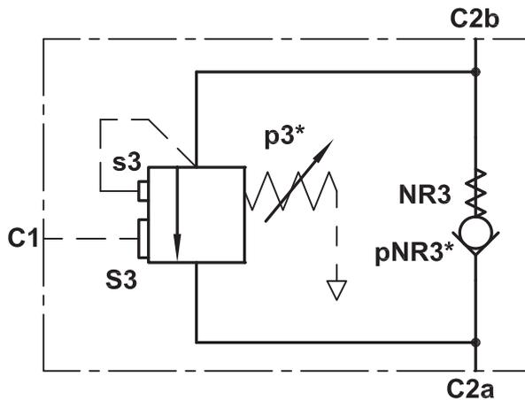
Fig. 10: ISO scheme of OVC3 valve
