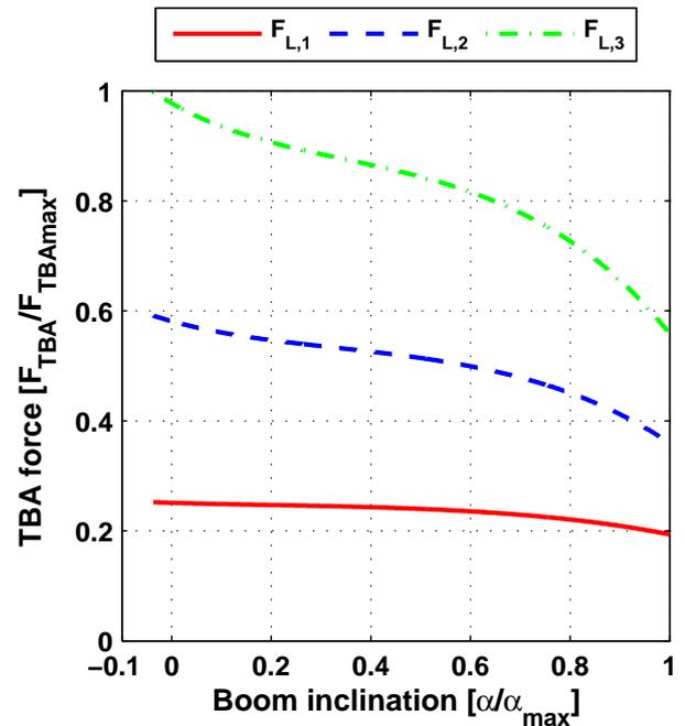
Fig. 8: Force  $F_{TBA}$  vs.  $\alpha$  for three values of  $F_{LOAD}$
