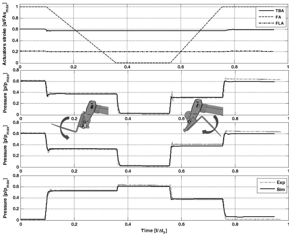
Fig. 26: FA bore side pressure  $P_1$  (top); Dual OVC C2a port pressure  $P_2$  (middle); FA rod chamber pressure  $P_3$  (bottom)
