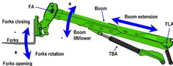
Fig. 2: Movements of telescopic boom and forks
