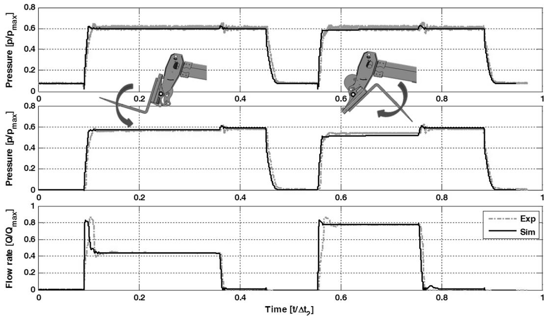
Fig. 27: Delivery pressure  $P_4$  (top); Load Sensing pressure  $P_5$  (middle); and delivery flow rate  $Q$  (bottom)
