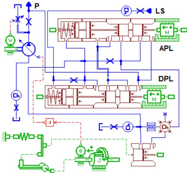
Fig. 17: AMESim pump model
