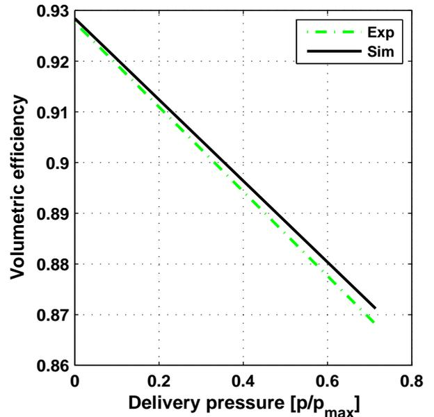
Fig. 18: Experimental vs. simulated pump volumetric efficiency at maximum pump displacement
