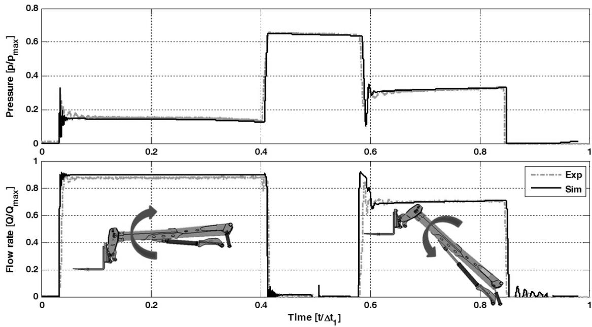
Fig. 25: TBA bore side pressure  $P_6$  (top); Delivery flow rate  $Q$  (bottom)
