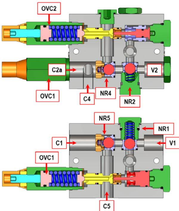
Fig. 13: Section views of OVC2 and OVC1
