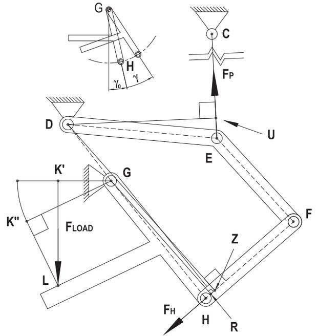
**Fig. 5:** Zoom of the forks handling system
