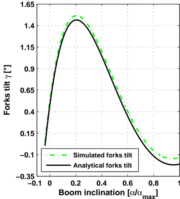
Fig. 23: Analytical vs. Simulated forks tilt
