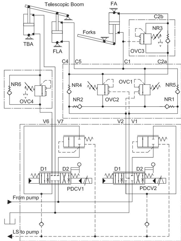
Fig. 3: The hydraulic circuit
