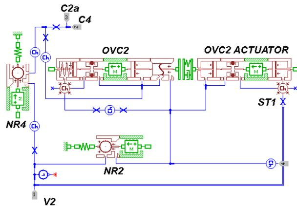
Fig. 15: Detailed model of the dual OVC valve
