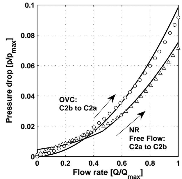
Fig. 12: Comparison between simulated and experimental pressure drop at maximum opening (For  $Q_{max}$  and  $p_{max}$  values refer to Table 2)
