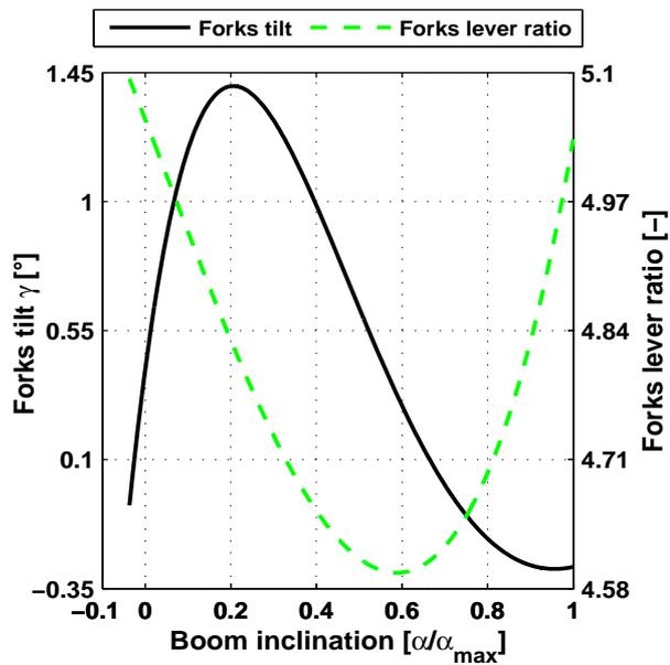
Fig. 7: Forks inclination and lever ratio
