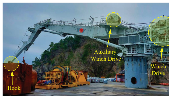
Figure 1 Offshore knuckle-boom crane from NOV placed on land. It is rated for loads up to 150 tons. Also shown in [6].
