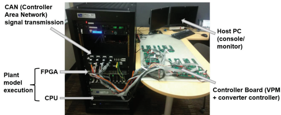
Figure 9 Image of the real HIL test rig.
