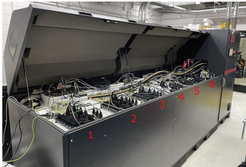
Figure 8 MTS HPU62 (6 bay DDP).
