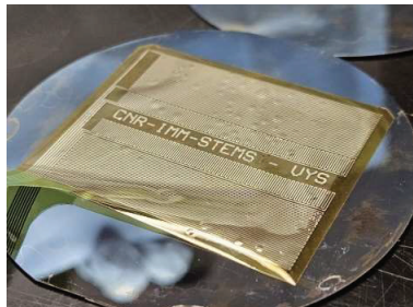
Figure 4 The ultra-thin device after the mechanical release from the wafer. On the left it is possible to see part of the adaptor with the routing for the four sensors.
