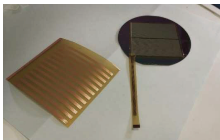
Figure 7 A photograph of the strain gauge with the adaptor.
