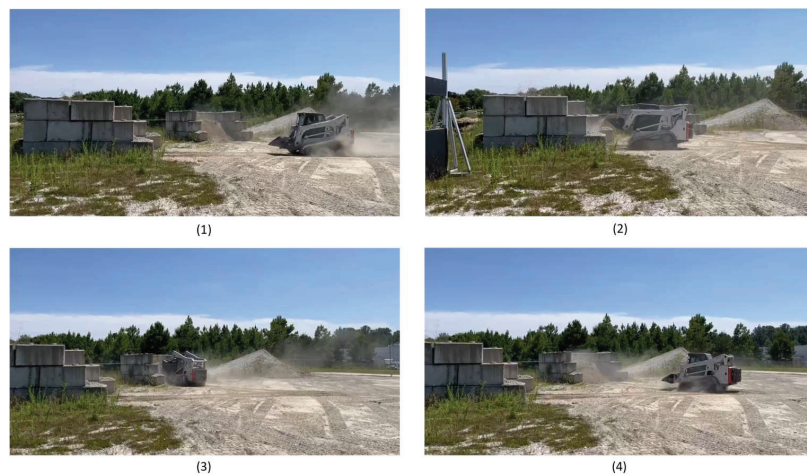
Figure 8 Y-cycle operation of the electrified compact track loader on the test field.
