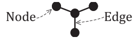
Figure 3 Example of an unlabeled connected graph with 4 nodes and 3 edges with designation of a node and an edge.
