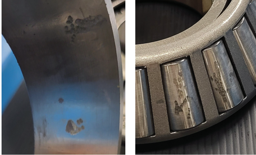
Figure 5 Examples for faulty roller bearings within the experimental test campaign. Left: Outer ring raceway. Right: Rolling elements.
