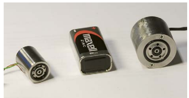
Fig. 7: Size comparison between the bistable hammer actuator on the left, a 9 V battery in the middle and the bistable valve presented in (Uusitalo, 2009) on the right
