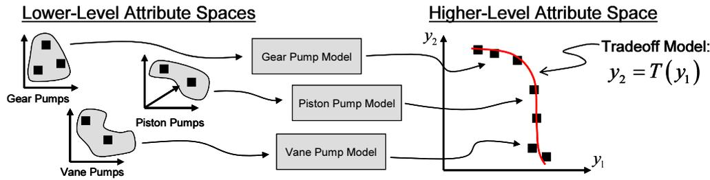
Fig. 1: Visualization of the distinction between tradeoff models and the models typically used for evaluating designs
