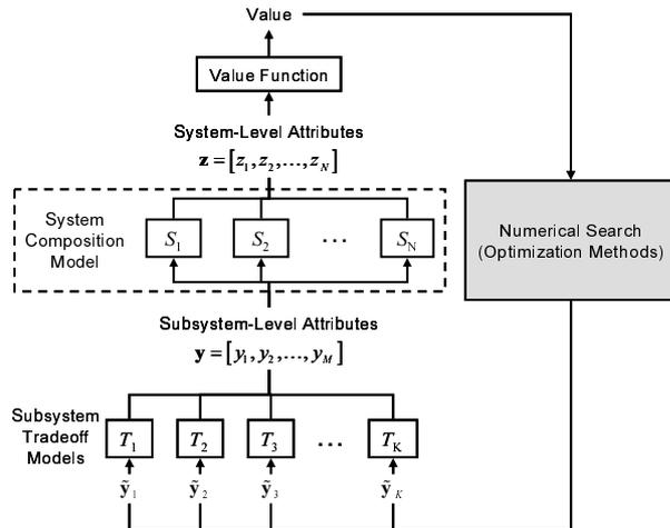
**Fig. 4:** Compositional modelling framework. Component attributes are mapped to system-level attributes via the system composition model
