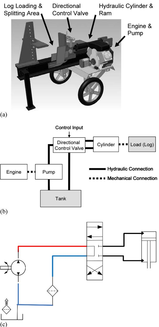
**Fig. 5:** Hydraulic log splitter: (a) physical layout, (b) functional configuration, where white boxes correspond to tradeoff models, and (c) circuit diagram
