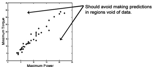
Fig. 3: Tradeoff model domain restrictions arising from the data
