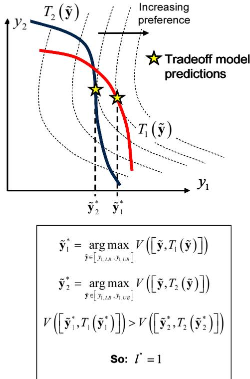
**Fig. 2:** Visualization of prediction and selection procedure using tradeoff models. The dashed curves are iso-preference curves
