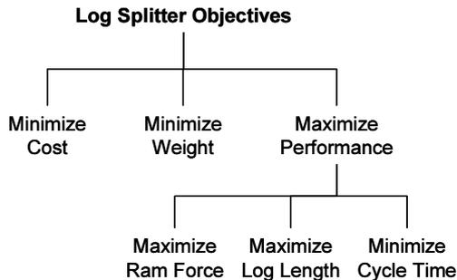
Fig. 6: Objectives hierarchy for the log splitter problem
