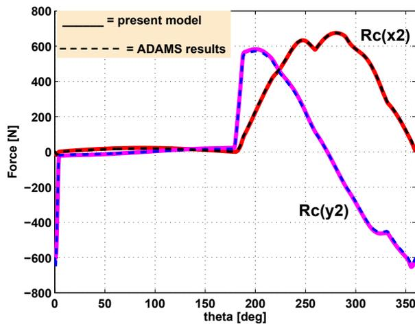
Fig. 27: Comparison on reactions Rc
