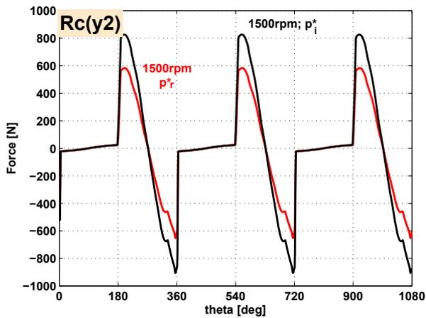
Fig. 20:  $R_c$  reaction, component  $y_2$
