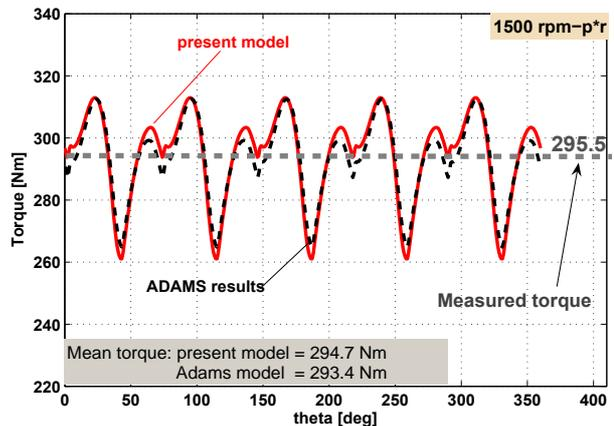
Fig. 30: Comparison of pump instantaneous and mean torque
