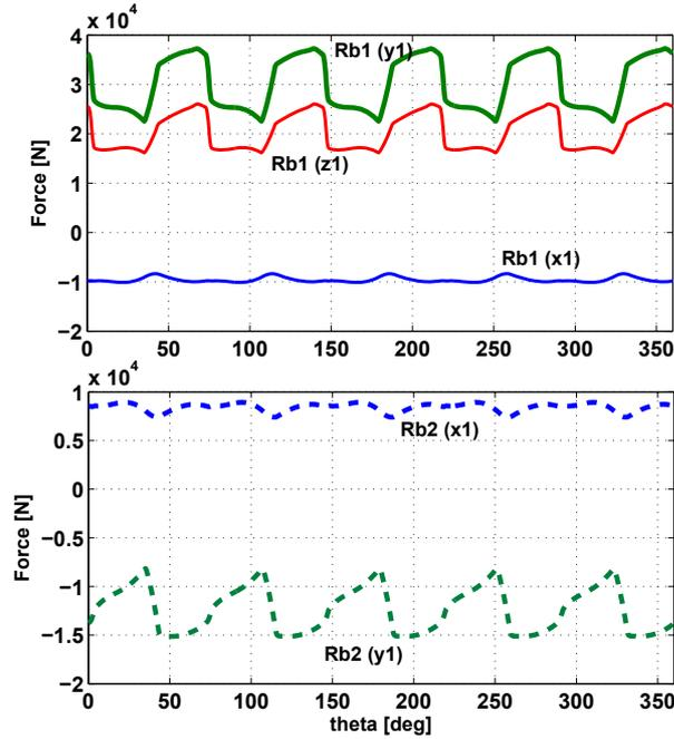
Fig. 15:  $R_{b1}$  and  $R_{b2}$  reactions (components) on shaft
