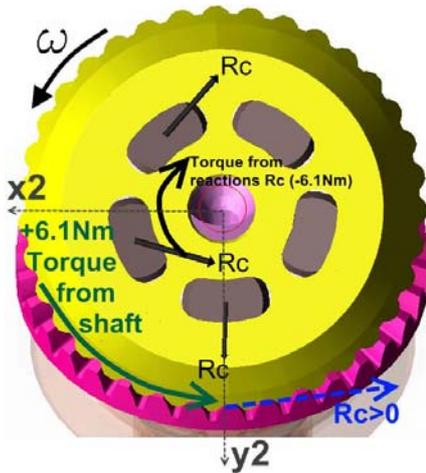
Fig. 31: Reactions  $R_c$ ,  $\vartheta = 0$
