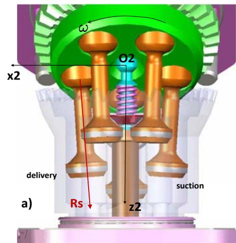
Fig. 13: Reaction  $R_s$ : plane  $x_2$ - $z_2$  and plane  $y_2$ - $z_2$
