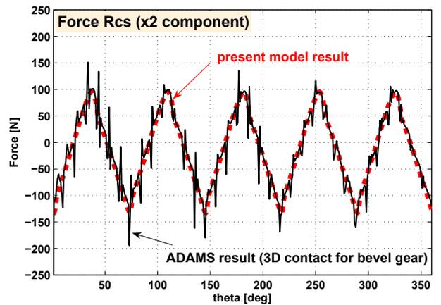
Fig. 34: Reaction cylinder block-shaft (present model and 3D contacts in ADAMS)
