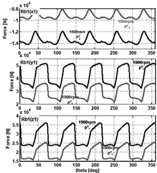
Fig. 23: Tapered roller bearing reactions ( $R_{b1}$ )
