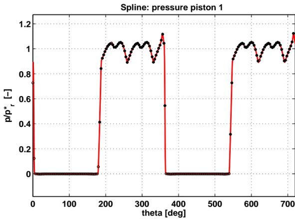
Fig. 25: Instantaneous pressure within a variable volume chamber (800 points for cubic spline, not all shown)
