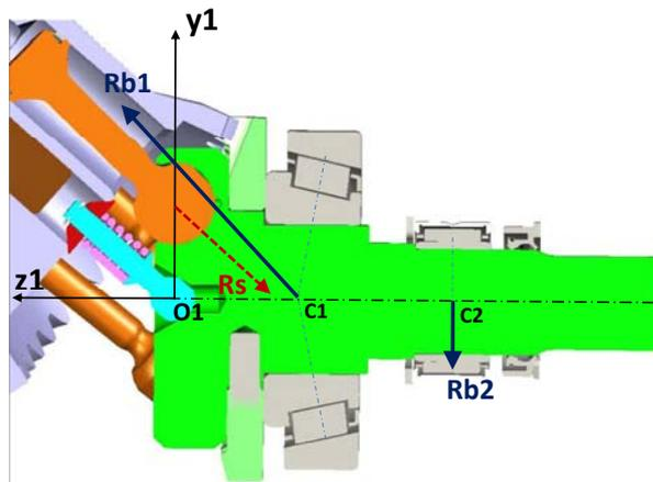
Fig. 16: Reactions on shaft from bearings
