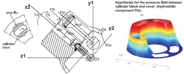
Fig. 8: cylinder block free body diagram
