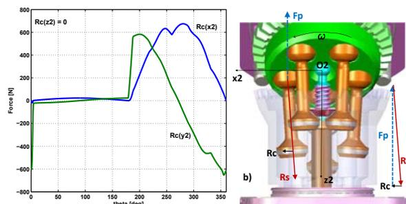
Fig. 14: Reactions  $R_c$  (components) and  $R_s$  (plane  $x_2$ - $z_2$ )
