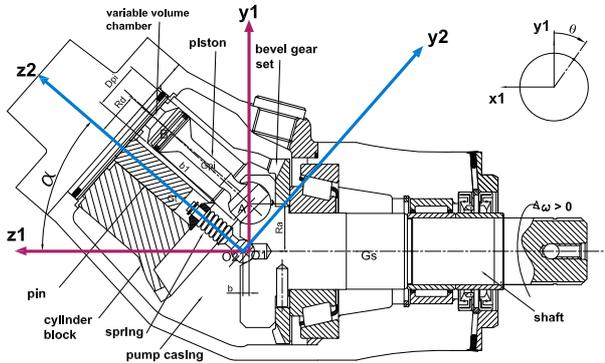
Fig. 1: Section view of the bent axis pump, coordinate systems and main geometric quantities
