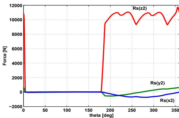
Fig. 12:  $R_s$ : piston-shaft reaction force
