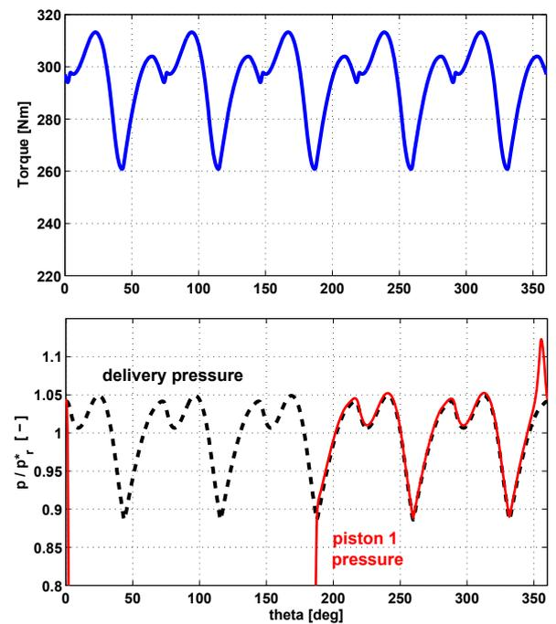
Fig. 17: Pump torque (top) and pressures (bottom)
