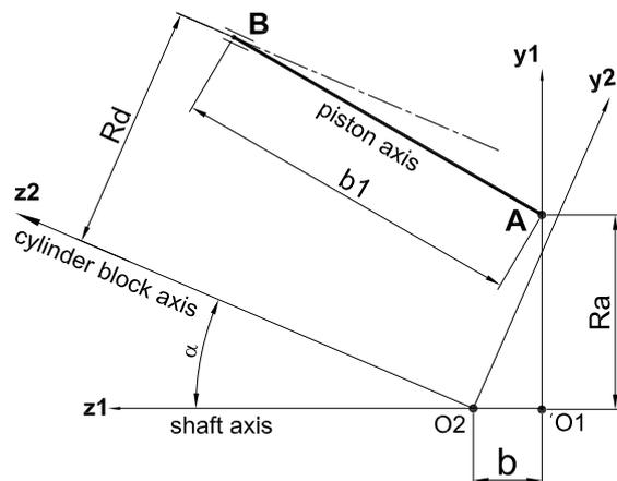
Fig. 3: Approach to pump kinematics
