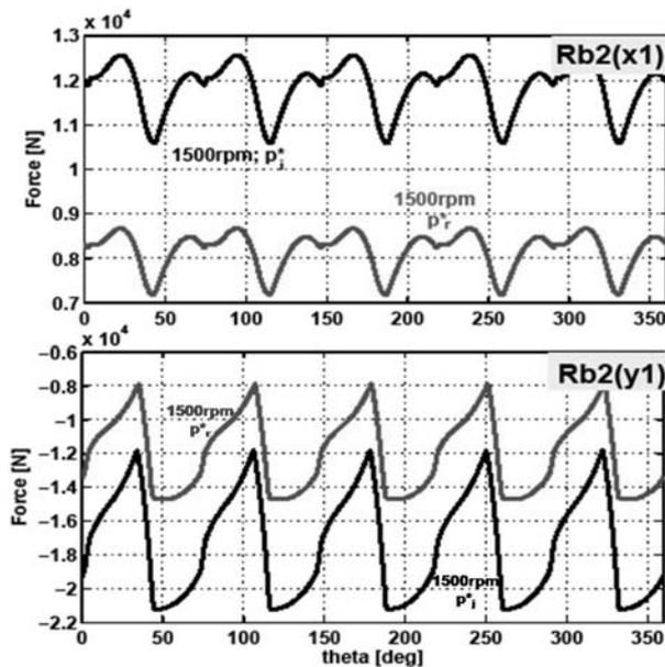
Fig. 24: Cylindrical bearing reactions ( $Rb2$ )
