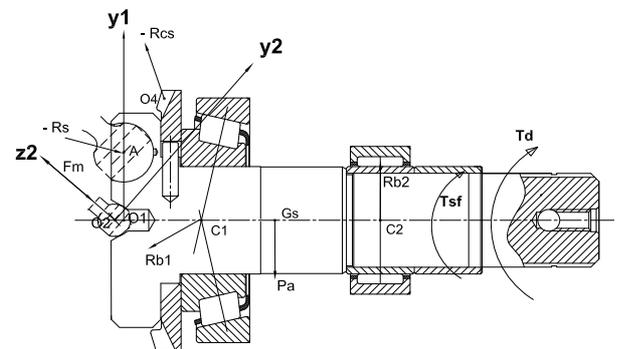
Fig. 7: Shaft free body diagram
