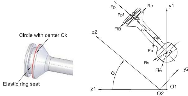
Fig. 6: Free body diagram of the piston
