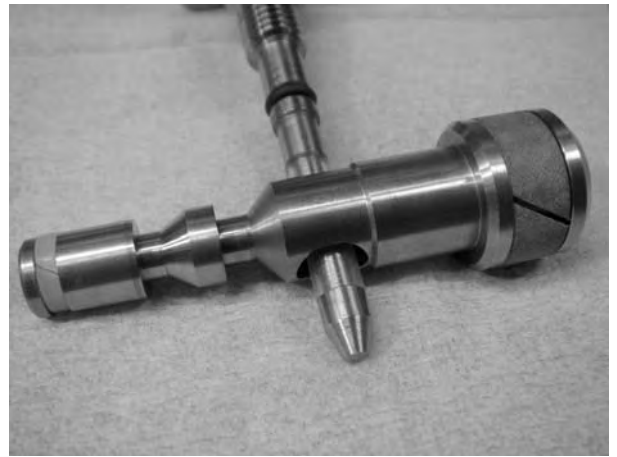
Fig. 4: The PC valve and the metering valve spindle
