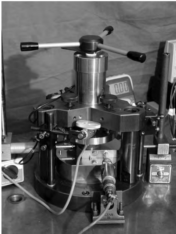
Fig. 5: Photo of the air pad test bed
