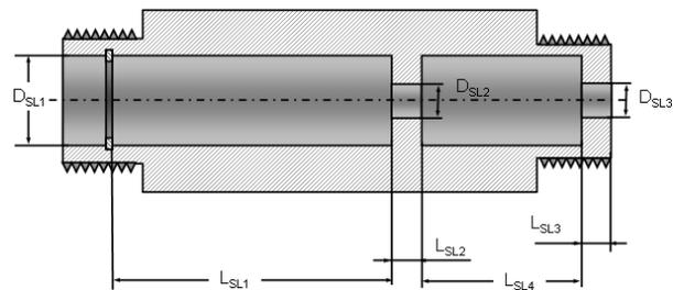
Fig. 4: Sleeve Critical Dimensions
