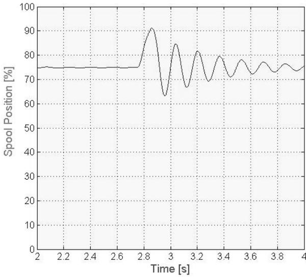
Fig. 32: Simulated spool position when switch from  $P_{load} = 150$  bar to  $P_T$
