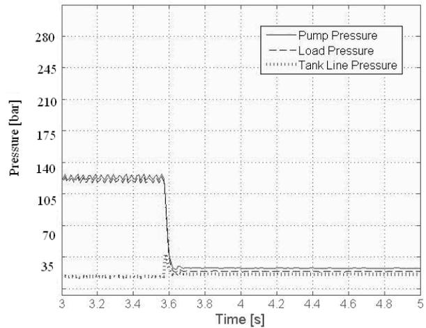
Fig. 24: Actual pressures when switch from  $P_{load} = 117$  bar to  $P_{tank}$
