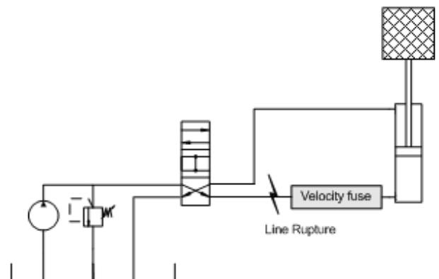
**Fig. 1:** Velocity fuse to protect subsystem
