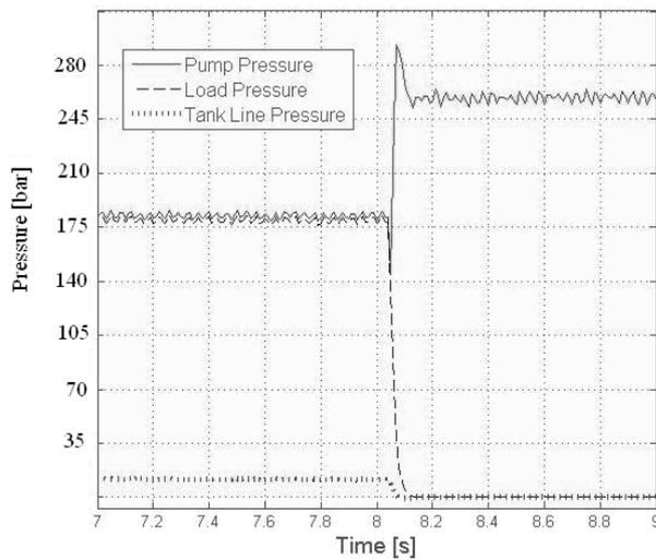
Fig. 39: Actual pressures when switch from  $P_{load} = 175$  bar to  $P_{atm}$
