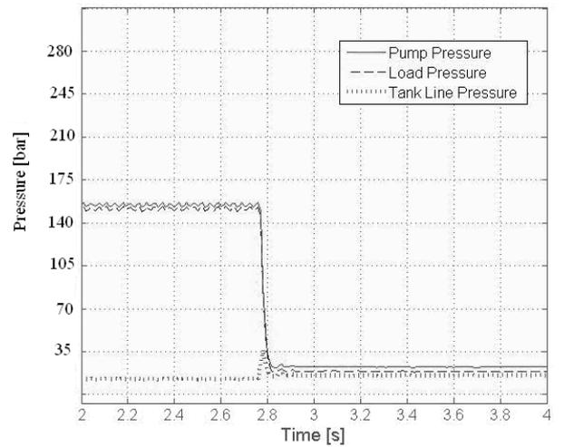
Fig. 30: Actual pressures when switch from  $P_{load} = 150$  bar to  $P_T$
