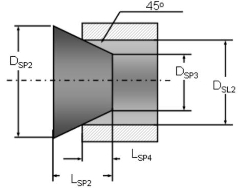
Fig. 10: Valve spool-sleeve geometrical relations
