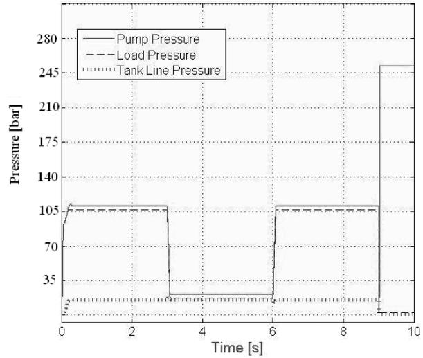
Fig. 16: Simulated pressures at  $P_{load} = 100$  bar
