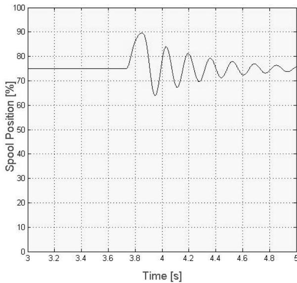
Fig. 38: Simulated spool position when switch from  $P_{load} = 175$  bar to  $P_T$
