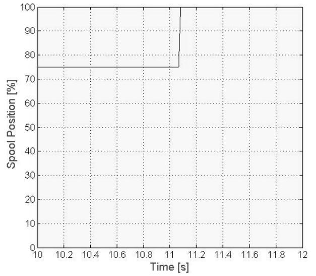
Fig. 29: Simulated spool position when switch from  $P_{load} = 117$  bar to  $P_{atm}$
