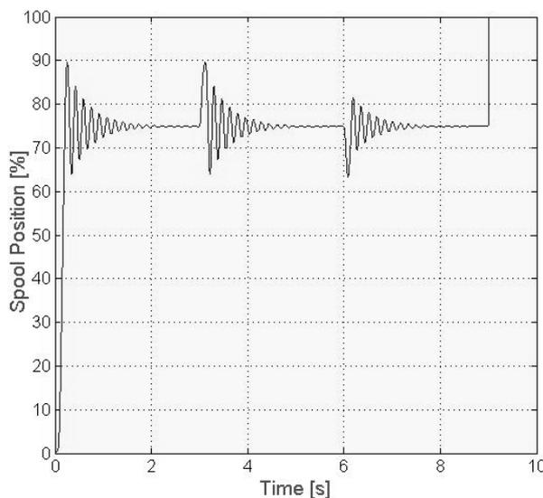
Fig. 21: Simulated spool position at  $P_{load} = 175$  bar
