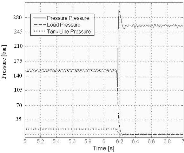
Fig. 33: Actual pressures when switch from  $P_{load} = 150$  bar to  $P_{atm}$
