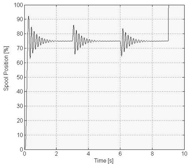
Fig. 17: Simulated spool position at  $P_{load} = 100$  bar
