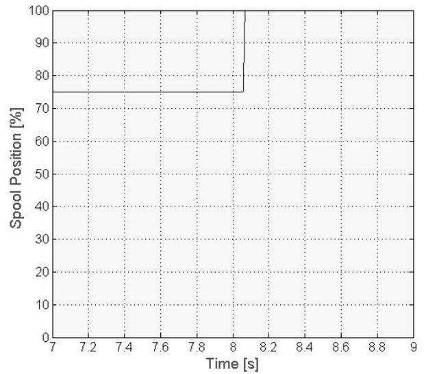
Fig. 41: Simulated spool position when switch from  $P_{load} = 175$  bar to  $P_{atm}$
