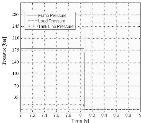
Fig. 40: Simulated pressures when switch from  $P_{load} = 175$  bar to  $P_{atm}$
