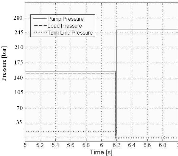
Fig. 34: Simulated pressures when switch from  $P_{load} = 150$  bar to  $P_{atm}$
