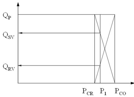
Fig. 15: Relief valve linear static characteristic
