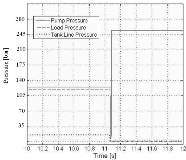
Fig. 28: Simulated pressures when switch from  $P_{load} = 117$  bar to  $P_{atm}$
