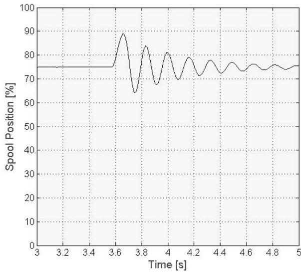
Fig. 26: Simulated spool position when switch from  $P_{load} = 117$  bar to  $P_T$
