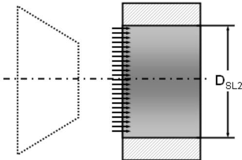
Fig. 14.a: Throttling area  $A_{23}$ , case 1
