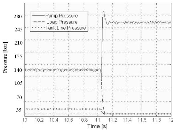
Fig. 27: Actual pressures when switch from  $P_{load} = 117$  bar to  $P_{atm}$
