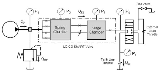
Fig. 13: Safety valve in the system
