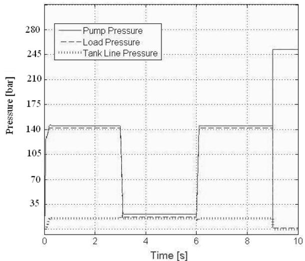
Fig. 18: Simulated pressures at  $P_{load} = 135$  bar
