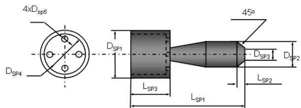
Fig. 5: Spool Critical Dimensions
