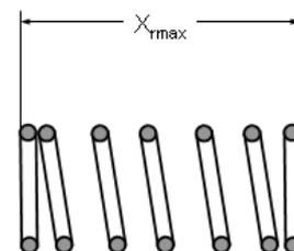
Fig. 6: Spring Critical Dimension
