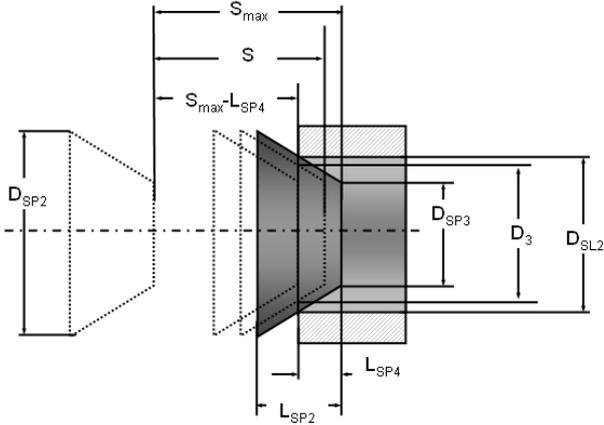
Fig. 12: Safety valve spool force balance
