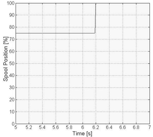
Fig. 35: Simulated spool position when switch from  $P_{load} = 150$  bar to  $P_{atm}$
