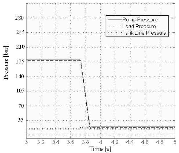
Fig. 37: Simulated pressures when switch from  $P_{load} = 175$  bar to  $P_T$
