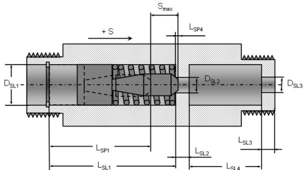
Fig. 9: Safety valve spool displacement
