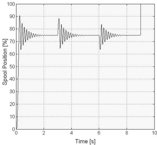
Fig. 19: Simulated spool position at  $P_{load} = 135$  bar
