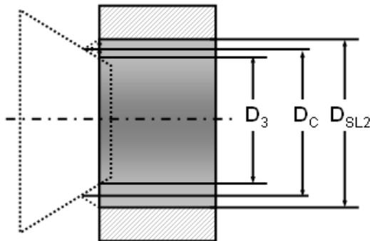
Fig. 14.b: Throttling area  $A_{23}$ , case 2
