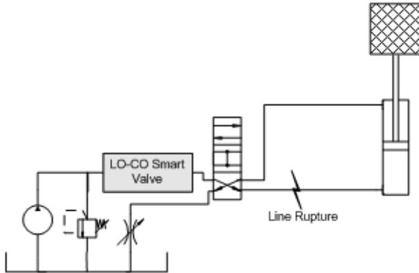
Fig. 2: Smart valve to protect the full system
