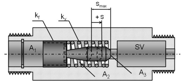
Fig. 11: Safety valve spool force balance
