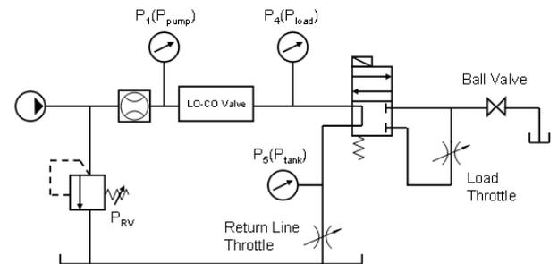
Fig. 22: Test hydraulic circuit
