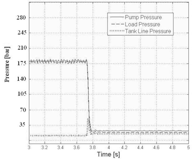
Fig. 36: Actual pressures when switch from  $P_{load} = 175$  bar to  $P_T$
