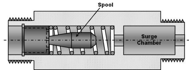
Fig. 3: Safety valve construction
