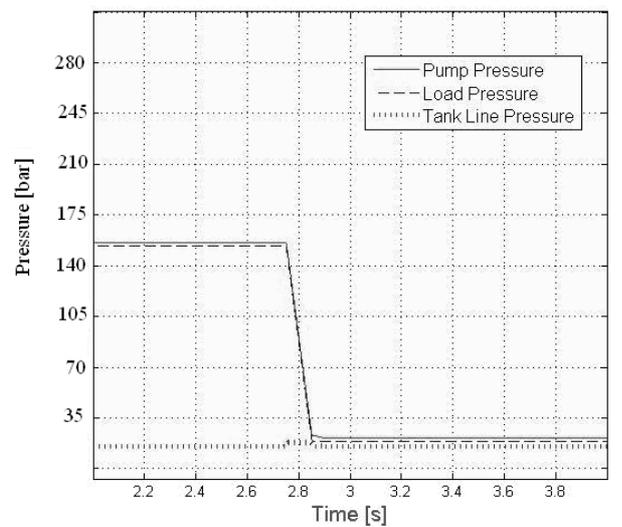
Fig. 31: Simulated pressures when switch from  $P_{load} = 150$  bar to  $P_T$
