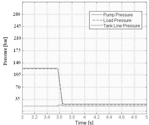
Fig. 25: Simulated pressures when switch from  $P_{load} = 117$  bar to  $P_T$
