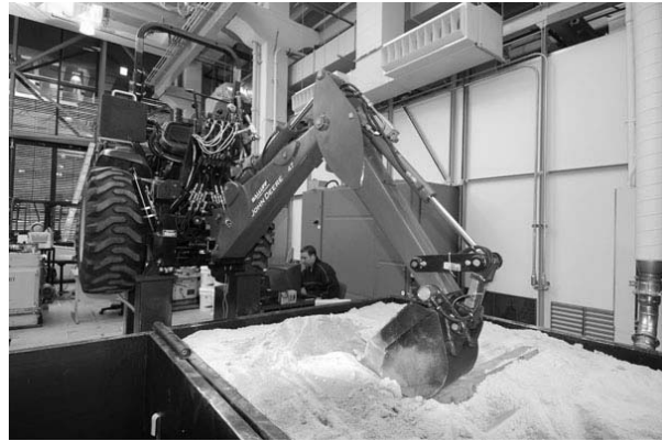
Fig. 1: Georgia Tech's haptic backhoe test-bed
