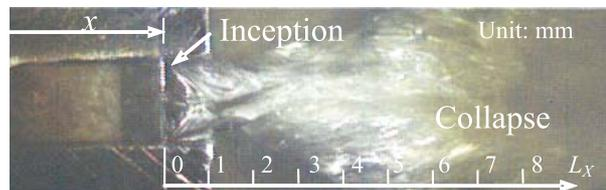
**Fig. 14:** Characteristic of cavitation appearance, IN
