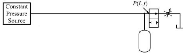
Fig. 15: Scheme of the studied system
