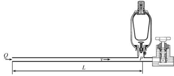
Fig. 14: Functional scheme of accumulator used for protection against pressure shocks
