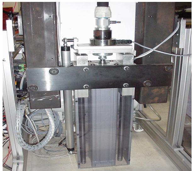
**Fig. 4:** Detail of the antagonist cylinder and of the load cell.
