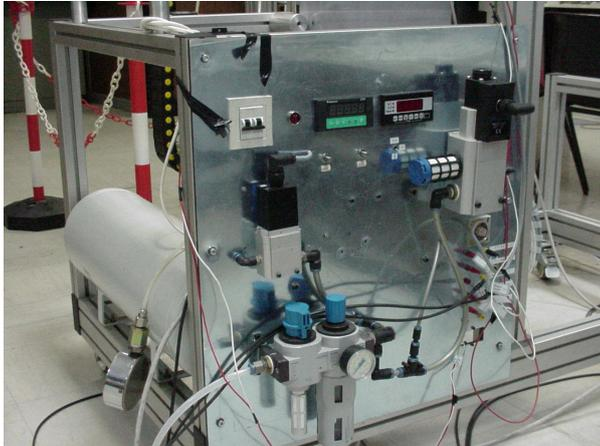
Fig. 5: Detail of pneumatic proportional valves.
