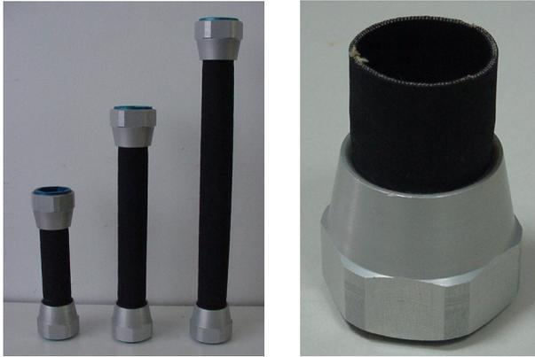
Fig. 1: Fluidic muscles and sectioned view
