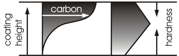
Fig. 5: Carbon content and hardness of a ZrC_g -coating
