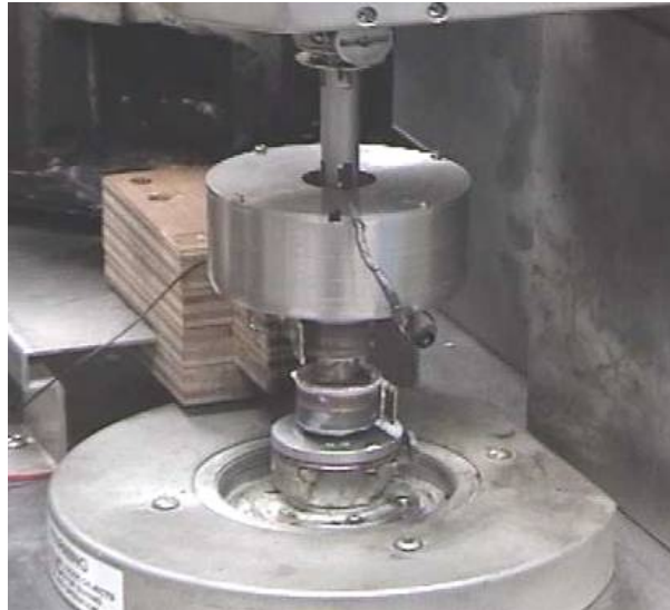
Fig. 1: Rheometer retrofitted with new MR test fixture.
