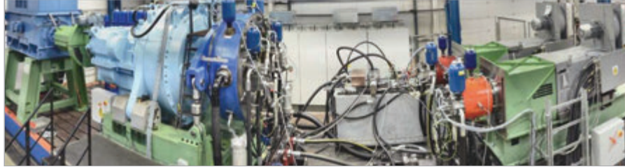
Figure 7 Panoramic view of the test-rig as built. Just right of centre is the (grey) backup oil reservoir. Partially out of sight in front of it are the two high-accuracy flow-meters.
