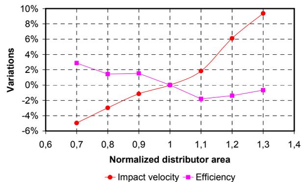
Fig. 14: Variations in impact velocity and efficiency depending on variations in the diameter  $D_{d2}$
