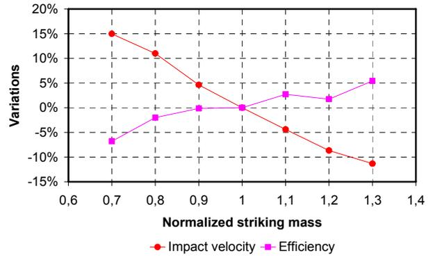
Fig. 7: Variations in impact velocity and efficiency depending on variations in mass of the piston
