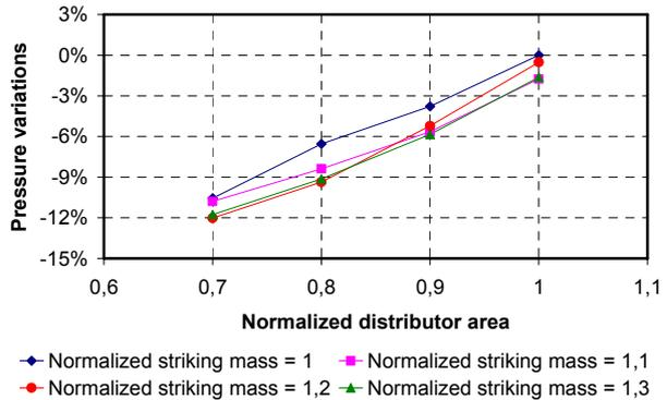
Fig. 17: Variations in working pressure with combined variations of piston mass and diameter  $D_{d2}$  of the distributor
