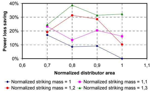
Fig. 16: Possibility of power saving with combined variations of piston mass and diameter  $D_{d2}$  of the distributor
