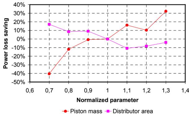
Fig. 15: Possibility of power loss saving with variations of the piston mass and of the diameter  $D_{d2}$  of the distributor
