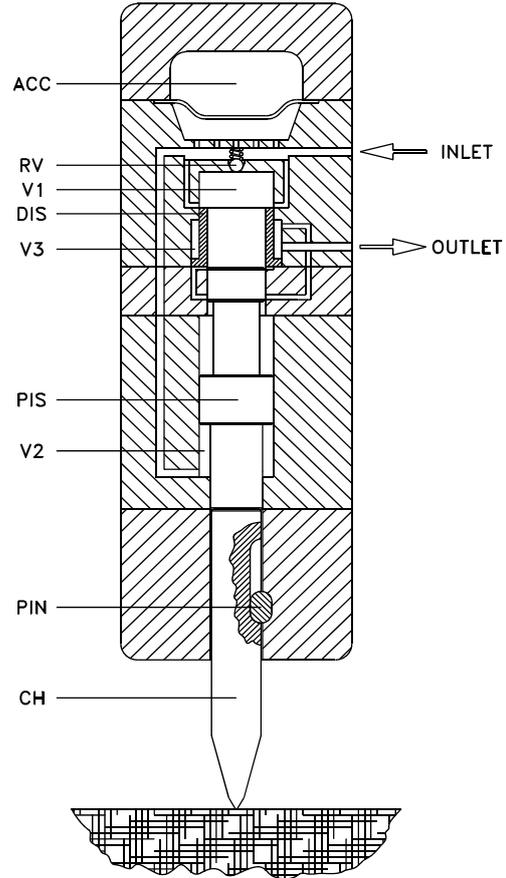
Fig. 1: Schematic drawing of the hydraulic breaker adapted from European Patent no. 0426928
