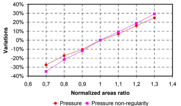
Fig. 8: Variations in working pressure and its non-regularity depending on variations in the areas ratio
