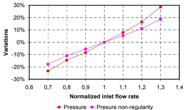
Fig. 4: Variations in working pressure and its non-regularity depending on variations in inlet flow rate
