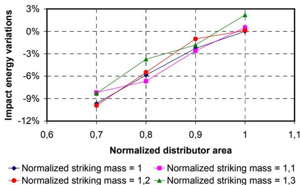
**Fig. 19:** Variations in impact energy with combined variations of piston mass and diameter  $D_{d2}$  of the distributor
