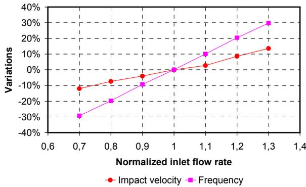
Fig. 5: Variations in impact velocity and working frequency depending on variations in inlet flow rate
