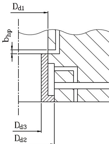
Fig. 12: Schematic drawing of the distributor ready to leave its bottom dead centre
