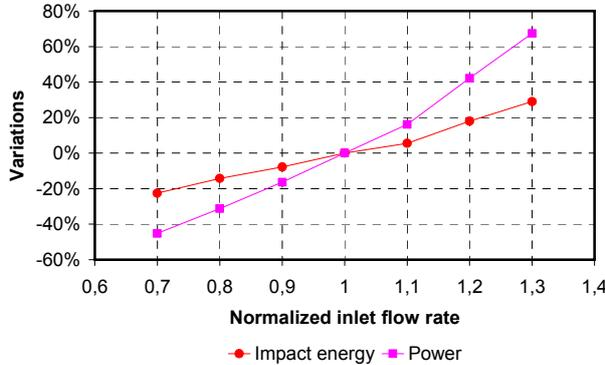
Fig. 6: Variations in impact energy and power depending on variations in inlet flow rate
