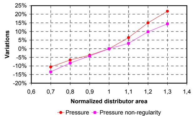
Fig. 13: Variations in working pressure and its non-regularity depending on variations in the diameter  $D_{d2}$
