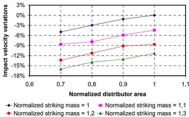
**Fig. 18:** Variations in impact velocity with combined variations of piston mass and diameter  $D_{d2}$  of the distributor
