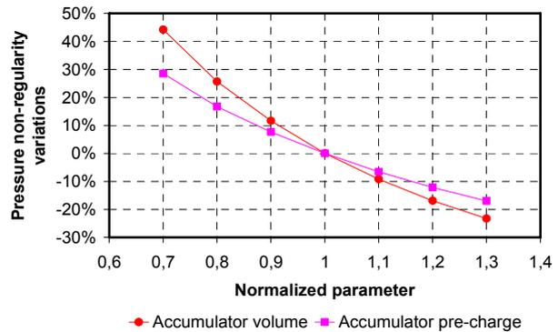
Fig. 11: Variations in pressure non-regularity at the inlet of the breaker depending on variations in volume and pre-charge of the accumulator
