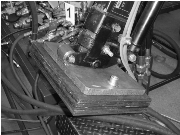
Fig. 16: Load on the crane end-effector (100 [kg])
