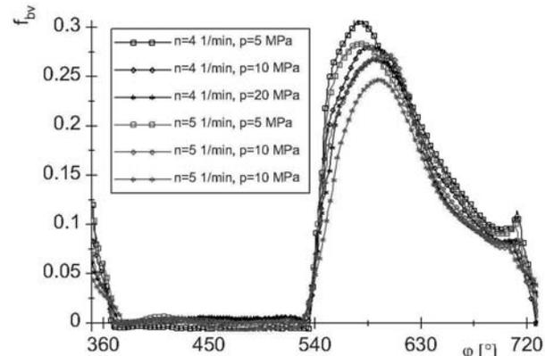
Fig. 19: Impact of pressure on the friction
