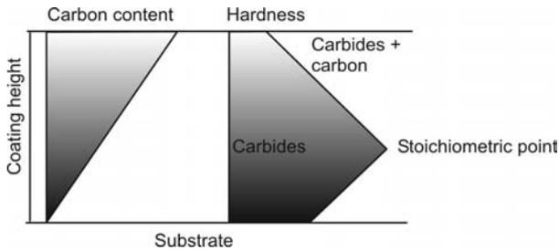
Fig. 1: Structure of the ZrC<sub>g</sub>-coating film
