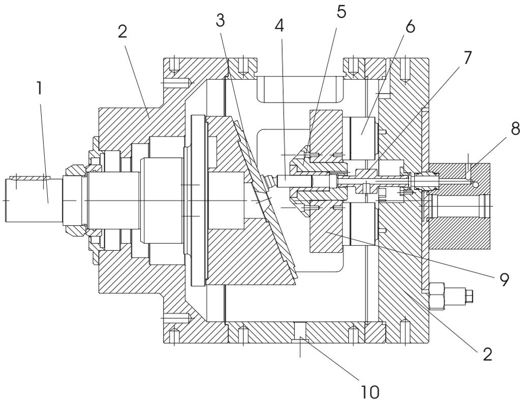
Fig. 7: Cross section of the test setup; 1: drive shaft, 2: housing, 3: swash plate in wobble design, 4: piston, 5: bushing (with singleserving worn inner part), 6: 4 piezo sensors, 7: compensation piston, 8: position for adapting a valveplate alternative, 9: plate, 10: exit for leakage
