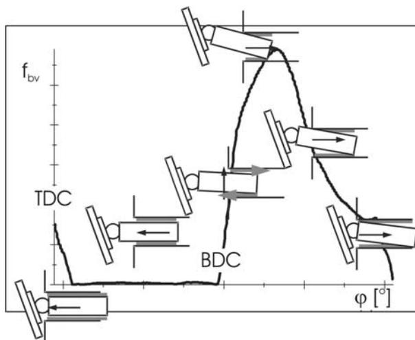
Fig. 10: Dislocation of the piston while moving in pump mode
