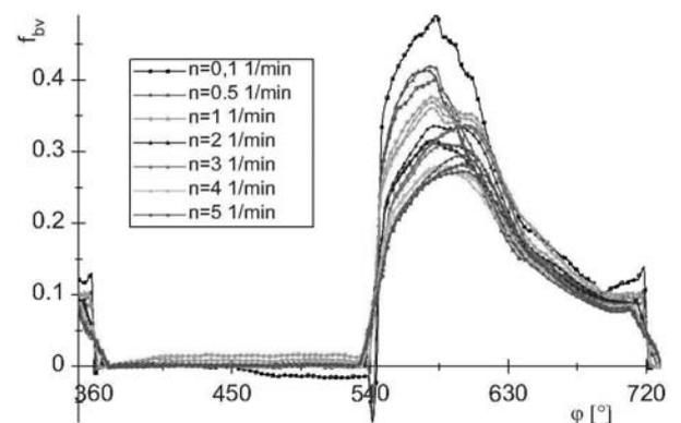
**Fig. 13:** Friction forces of the cylindrical piston in pump mode at  $p = 10$  MPa
