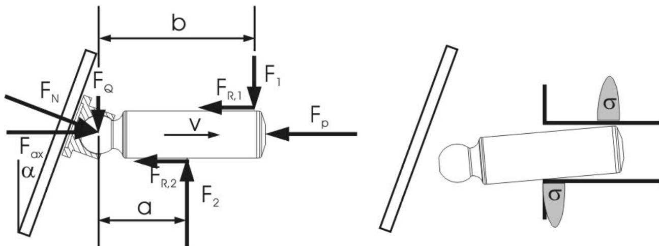
Fig. 2: Static balance of forces at the inclined piston in pump mode
