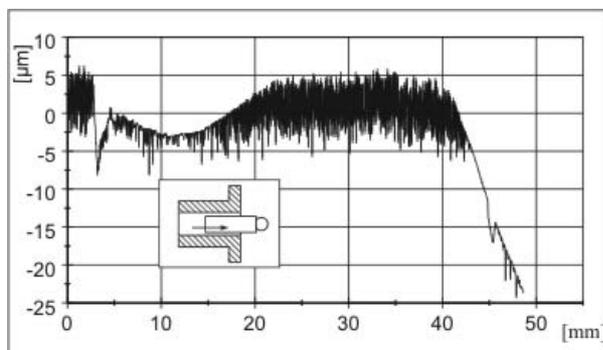
Fig. 20a: Profil of the piston with reduced diameter
