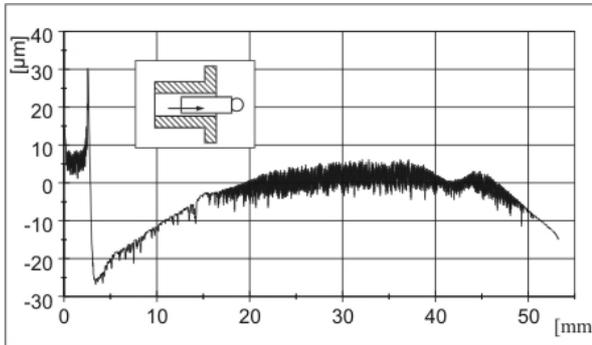
Fig. 14b: Profil of the bushing
