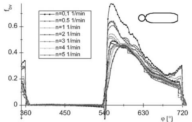
Fig. 21: Friction of a piston with reduced diameter in pump mode at  $p = 10 \text{ MPa}$
