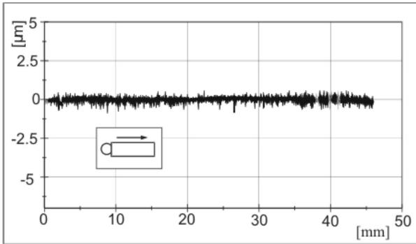
Fig. 14a: Profil of the industrial piston
