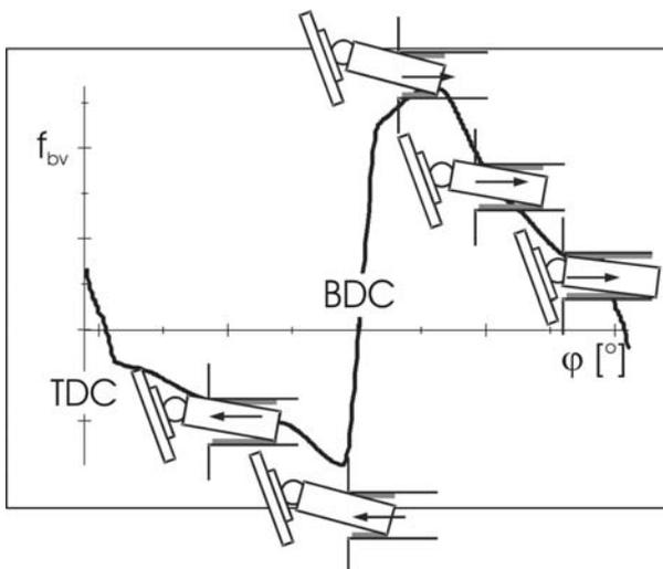
**Fig. 12:** Dislocation of the piston while moving in pump-motor mode
