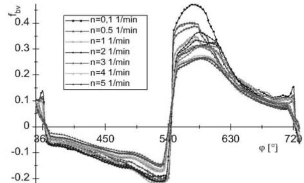
Fig. 17: Friction forces of the cylindrical piston in motor pump-mode at  $p = 10 \text{ MPa}$
