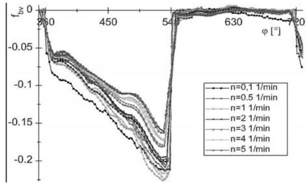
Fig. 16: Friction forces of the cylindrical piston in motor mode at  $p = 10 \text{ MPa}$
