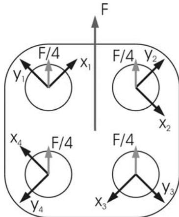
Fig. 9: Assembly of the piezo sensors in the  $x$ - $y$ -plane
