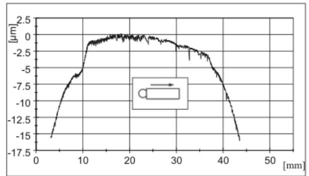
Fig. 20b: Profil of the bushing
