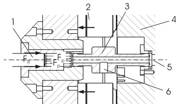
**Fig. 8:** 1: end of piston, 2: piezo sensor, 3: compensation piston, 4: housing, 5: position for adapting a valve-plate alternative, 6: access for pressure sensor,  $F_p$ : pressure force,  $F_f$ : friction force
