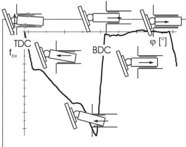
**Fig. 11:** Dislocation of the piston while moving in motor mode
