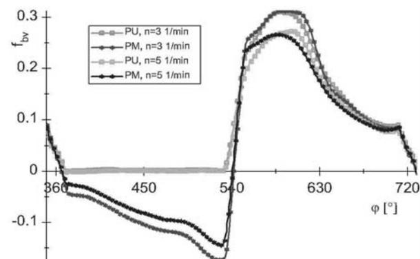
Fig. 18: Comparison of  $f_{bv}$  with and without squeeze effect at different numbers of revolution for  $p=10 \text{ MPa}$
