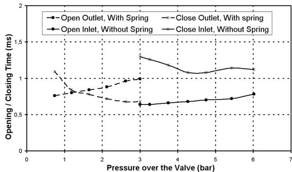
Fig. 7: Opening times and closing times of valves – when using PPAM between 0 and 3 bar
