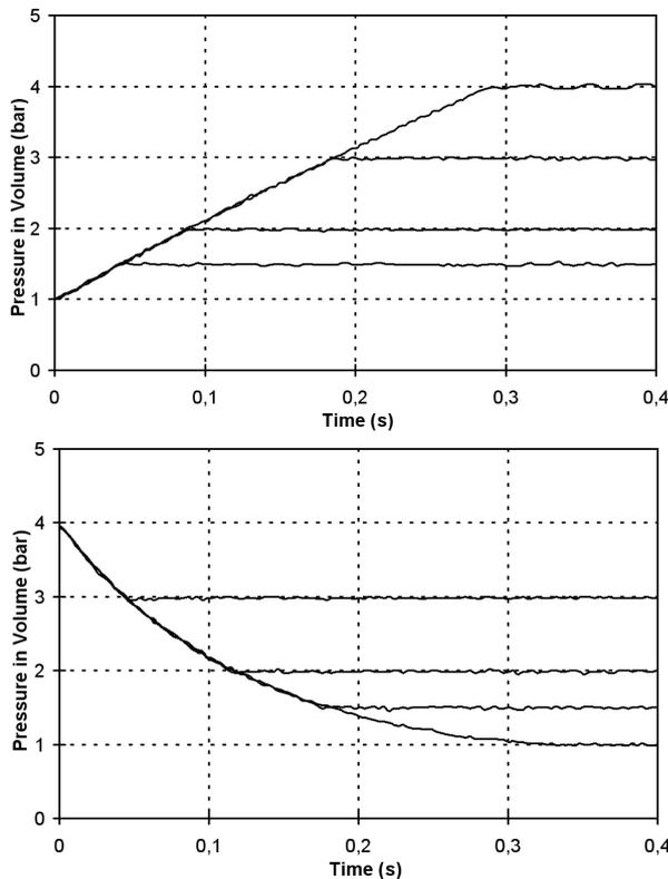
Fig. 9: Pressure Control (Increasing and decreasing pressure)
