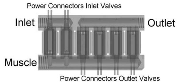
Fig. 10: Sliced view of the complete pressure control valve island with 2 inlet and 4 outlet valves
