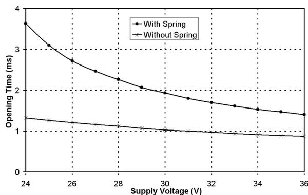
**Fig. 4:** Influence of supply voltage on the opening time of the valves,  $\Delta p=4.6$  bar
