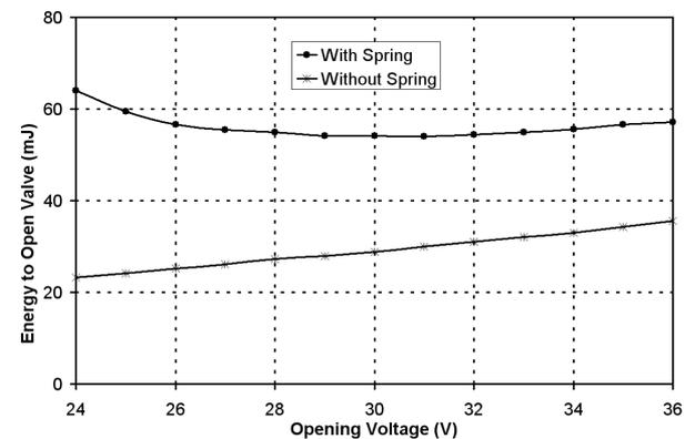
**Fig. 5:** Influence of supply voltage on energy to open valve,  $\Delta p=4.6$  bar
